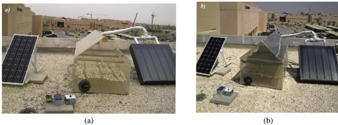
Fig. 5 Greenhouse attached with flat-plate collector and PV panel (a) without thermal curtain and (b) with thermal curtain
