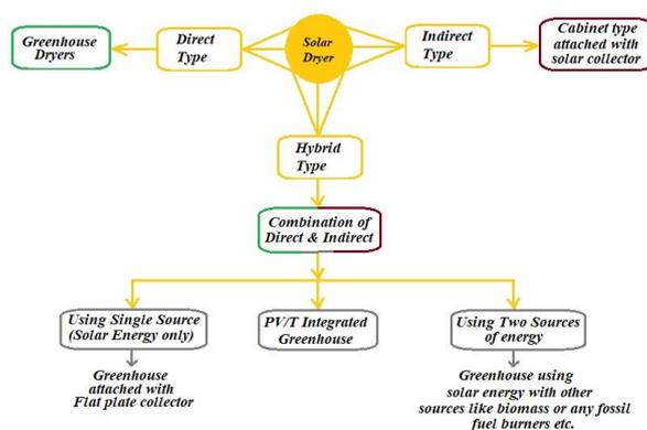
Fig. 2 Methods used for making greenhouse hybrid
