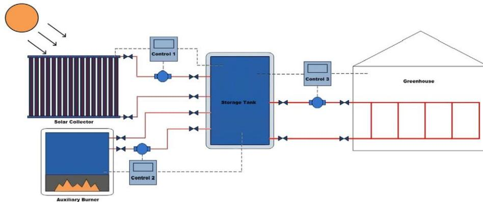
Fig. 12 The schematic diagram of proposed hybrid dryer
