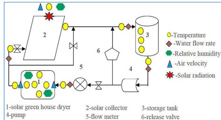
Fig. 10 Block diagram of proposed hybrid setup
