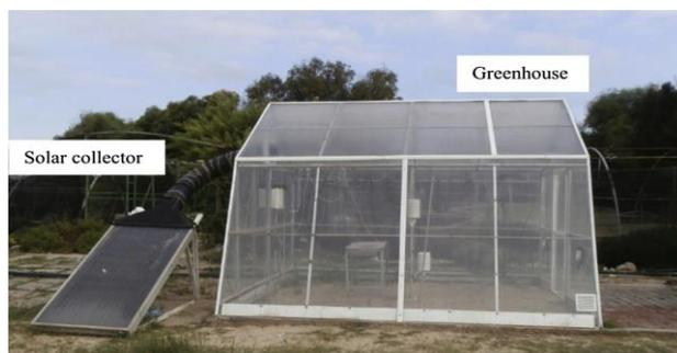
Fig. 6 Greenhouse dryer attached with flat plate collector
