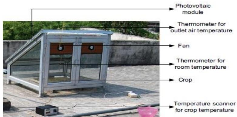
Fig. 4 The pictorial view of developed HGSD
