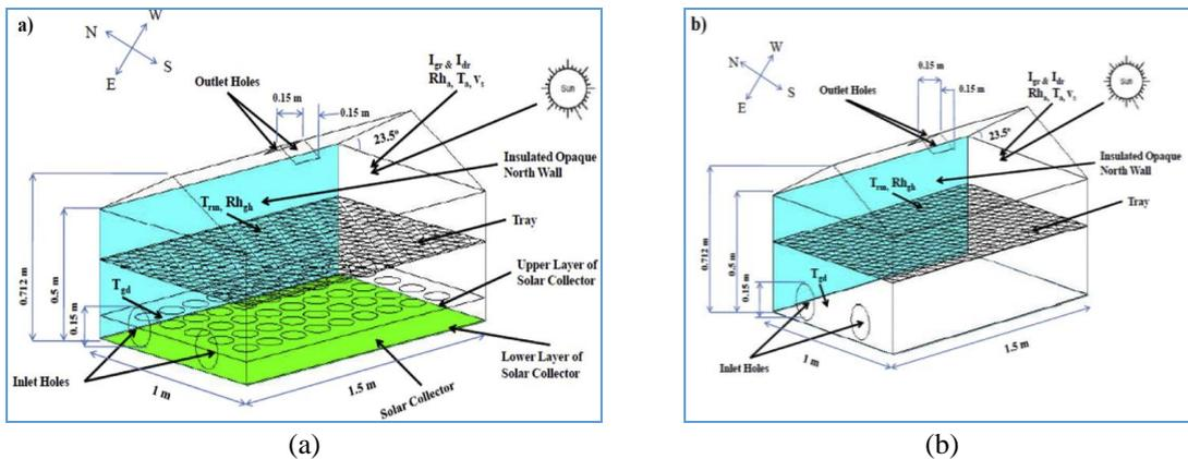
Fig. 9 Schematic representation of HGSD (a) with collector and (b) without collector
