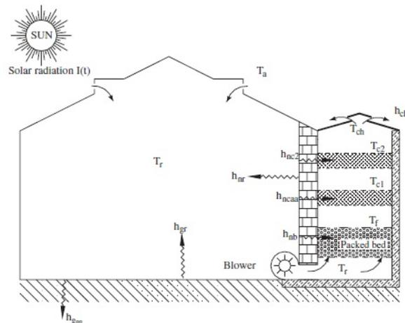
Fig. 13 The schematic view of greenhouse with separate drying chamber
