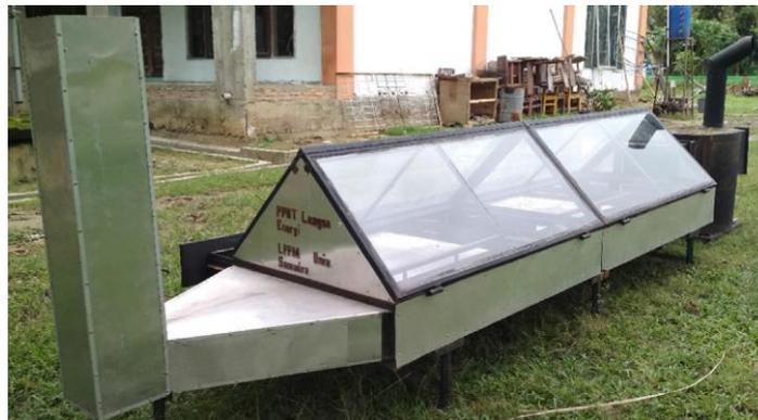
Fig. 11 The fabricated HGSD attached with biomass burner
