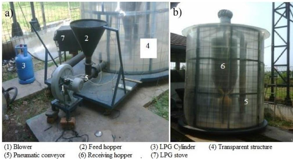
(1) Blower (2) Feed hopper (3) LPG Cylinder (4) Transparent structure
