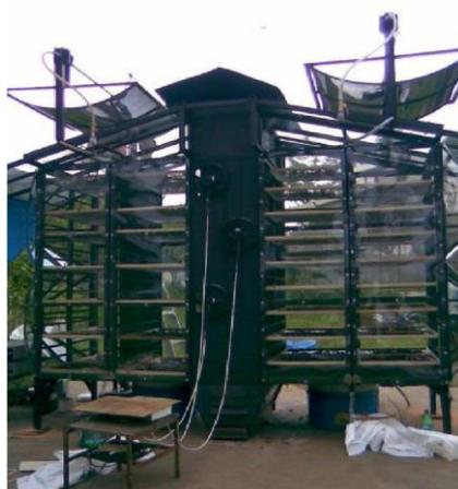
Fig. 15 Rack-type greenhouse attached with biomass burner
