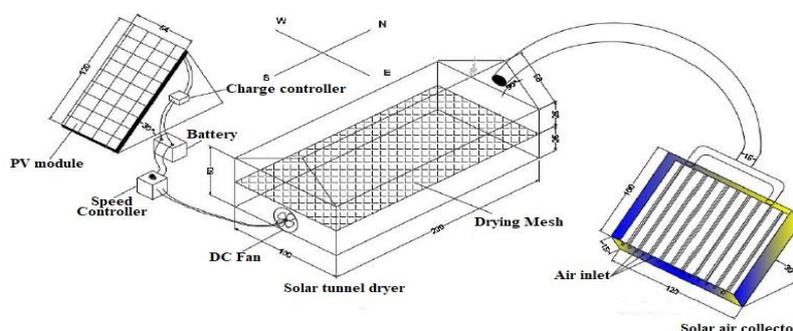
Fig. 7 Schematic diagram of greenhouse attached with solar collector and PV module
