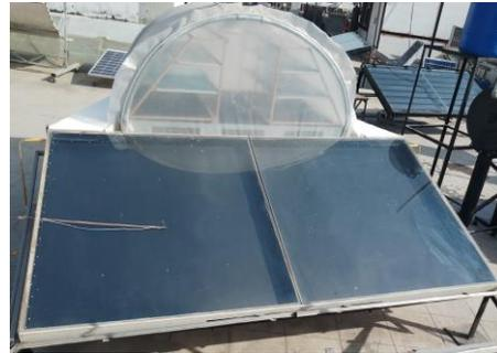
Fig. 8 Rack-type HGSD attached with flat-plate collector
