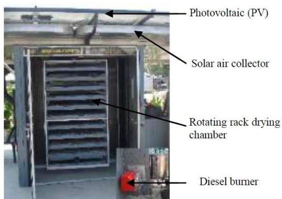
Fig. 14 Hybrid greenhouse attached with diesel burner
