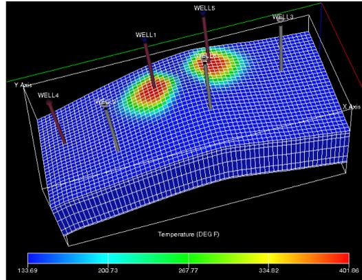
Fig. 1 3D dynamic model: reservoir temperature and wells system
