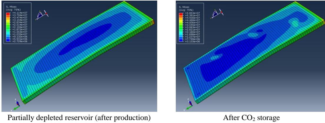
Fig. 12 Mises stress distribution
