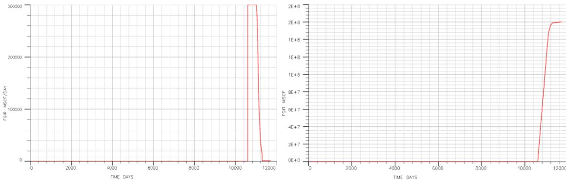
Fig. 9 Reservoir CO<sub>2</sub> injection rate (left), and cumulative injection volume (right)
