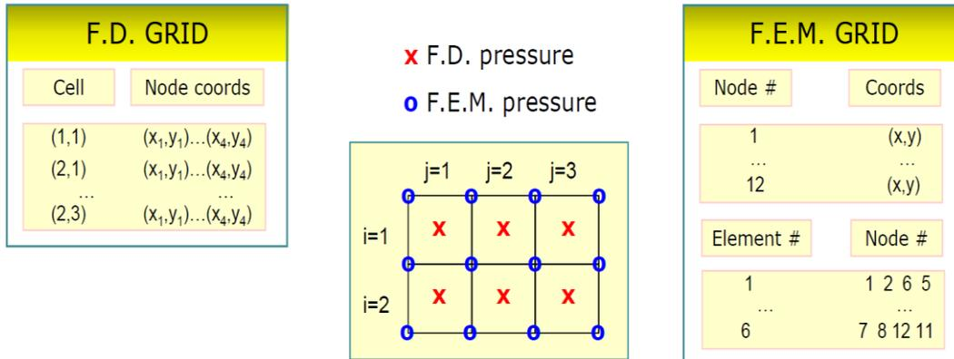
Fig. 5 Adjustment of finite difference and finite element mesh
