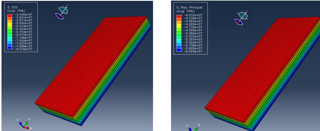
Fig. 10 Vertical stress (left), and maximum principal stress (right) distribution
