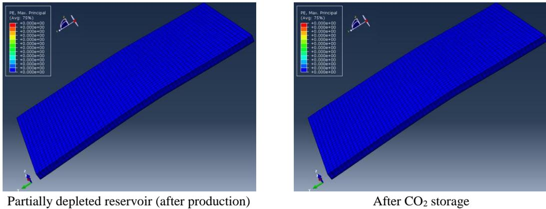
Fig. 13 Maximum plastic strain
