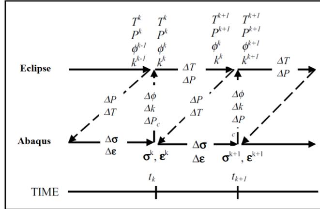
Fig. 4 Explicit sequential solutions of a linked ECLIPSE and ABAQUS simulation
