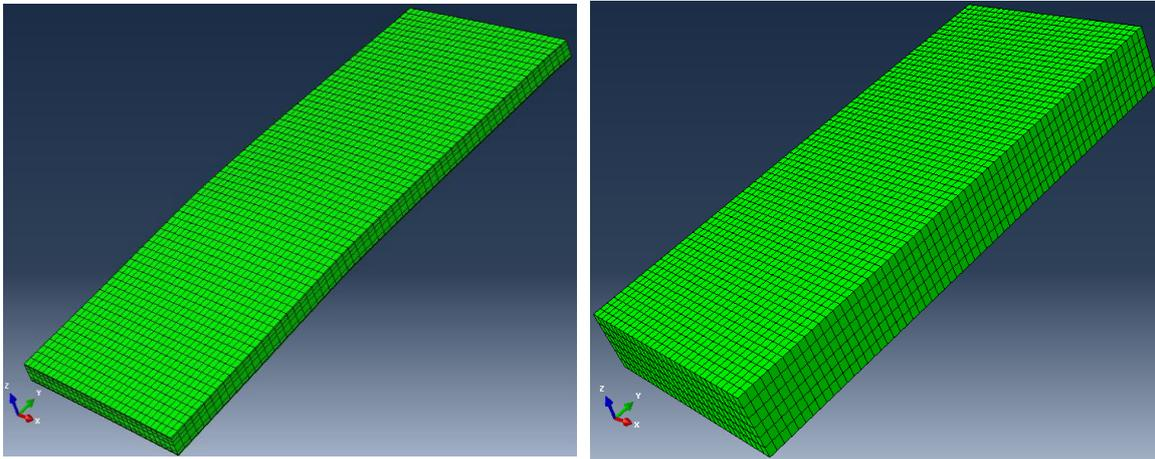
Fig. 2 3D geomechanical model: reservoir (left), and reservoir and its surrounding (right)
