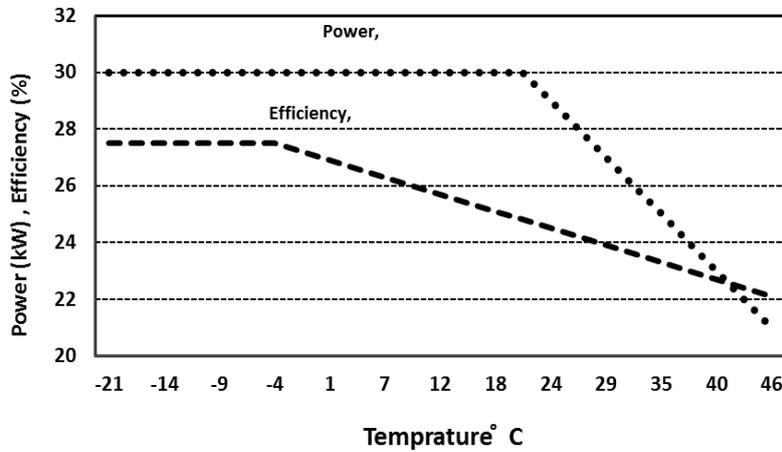
Fig. 7 Changes of e power and  $\eta$  efficiency in Capston C30 microturbine, considering the ambient temperature (www.capstonmicroturbine.com)
