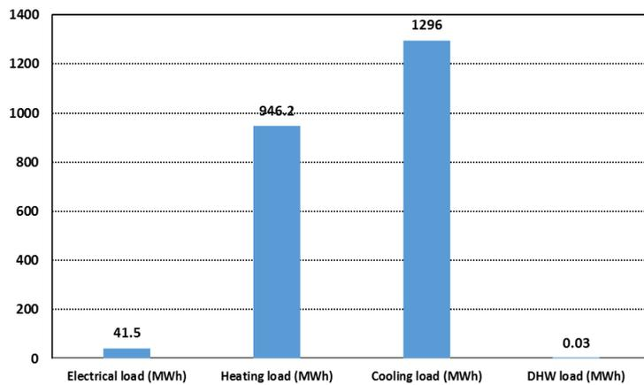
Fig. 8 Diagram of annual consumption of electrical, heating, cooling and DHW loads
