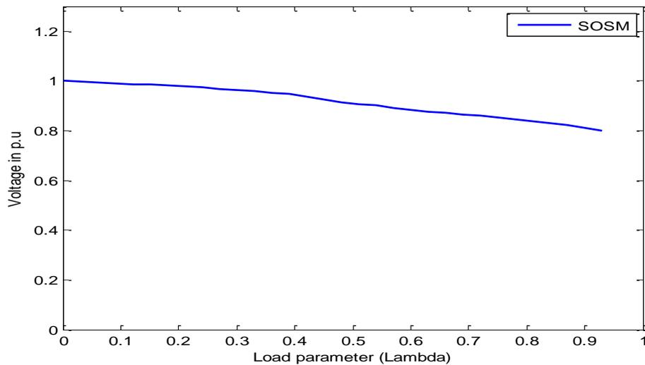
Fig. 8 P-V curve of the weakest bus (only taps) for multi-objective case
