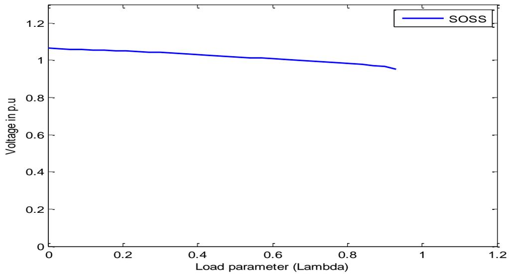
Fig. 13 P-V curve of the weakest bus (simultaneous) single objective case
