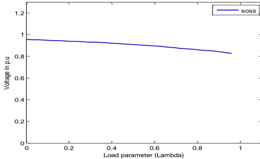
Fig. 10 P-V curve of the weakest bus (sequential UPFC) for single objective case
