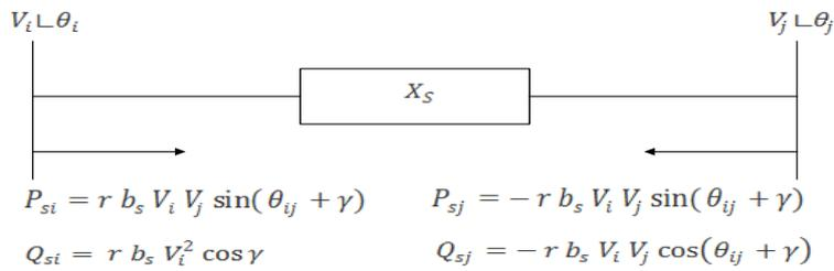
Fig. 3 UPFC injection model
