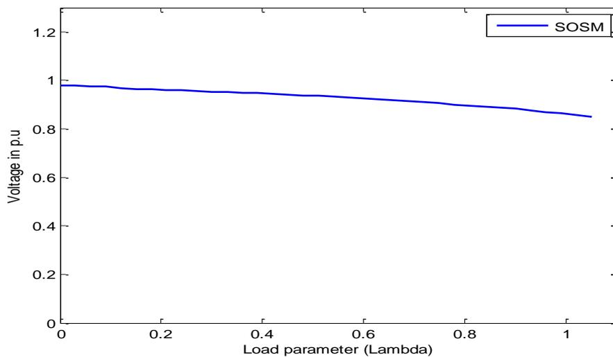
Fig. 11 P-V curve of the weakest bus (sequential UPFC) for multi-objective case
