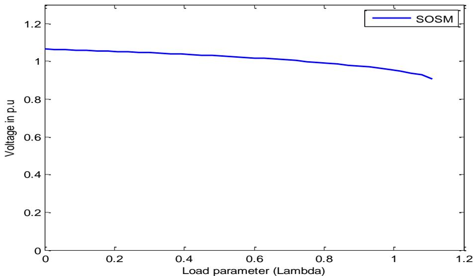
Fig. 14 P-V curve of the weakest bus (simultaneous) multi-objective case
