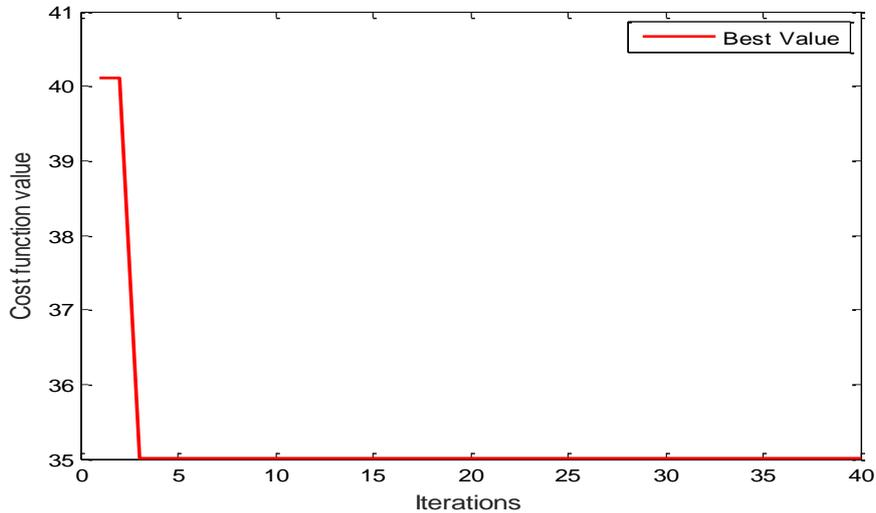
Fig. 9 Performance of SOS algorithm (sequential UPFC) for single objective case
