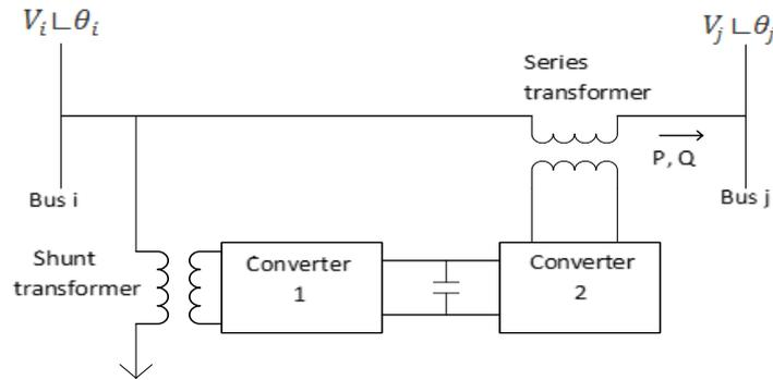
Fig. 2 UPFC device basic arrangement
