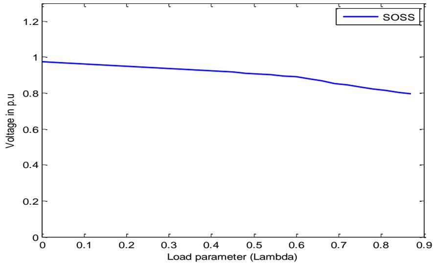
Fig. 7 P-V curve of the weakest bus (only taps) for single objective case
