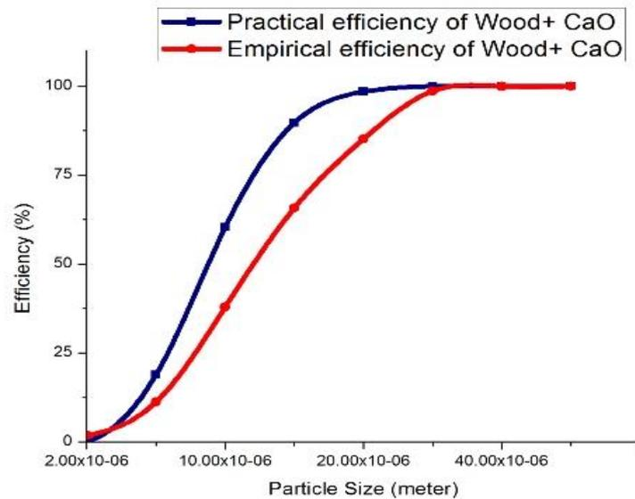
Fig. 8 Efficiency comparisons experimentally v/s Empirical model for feed stock Wood+CaO
