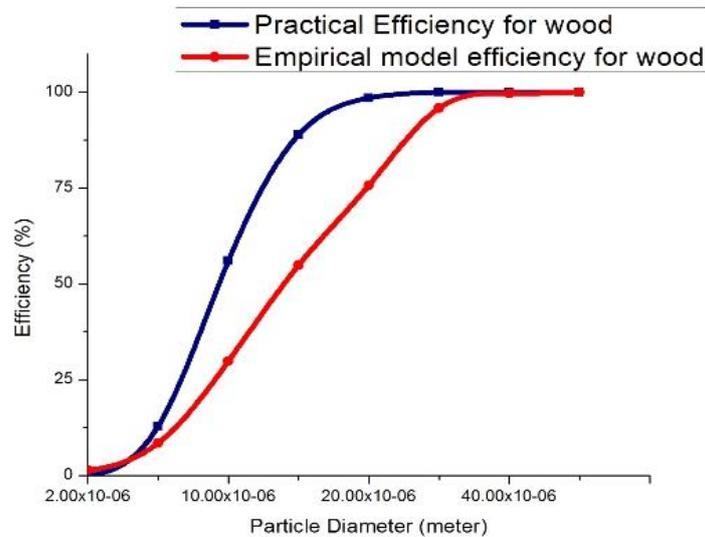
Fig. 7 Efficiency comparisons experimentally v/s Empirical model for feed stock Wood (Particle size efficiency for Wood Particle dia. in (m))
