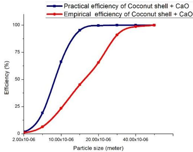
Fig. 10 Efficiency comparisons experimentally v/s Empirical model for feed stock Coconut shell+CaO
