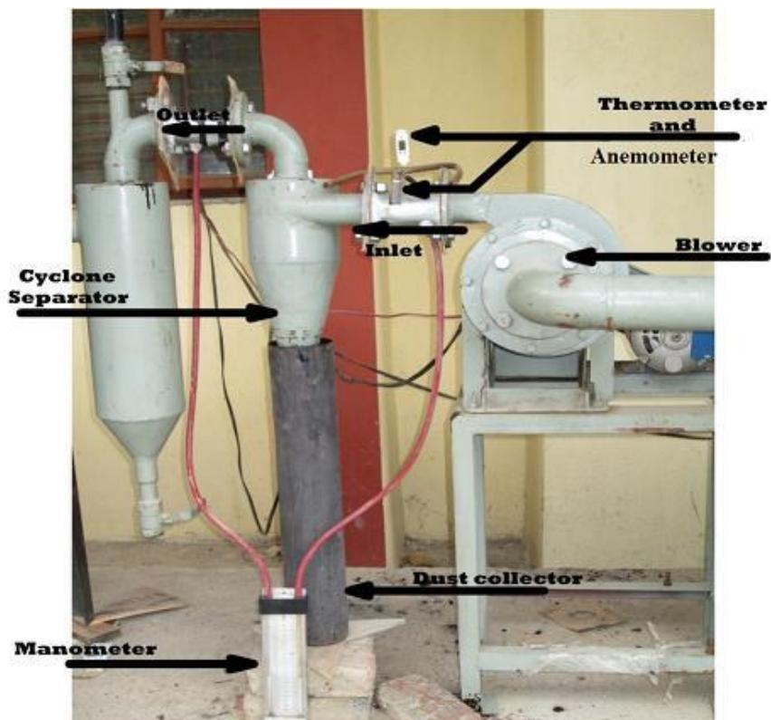
Fig. 3 Experimental setup at IIT (BHU)
