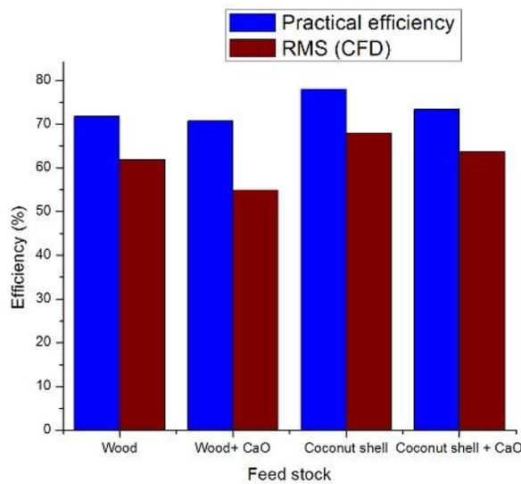
Fig. 11 Comparison of values of efficiency using RSM and conventional methods
