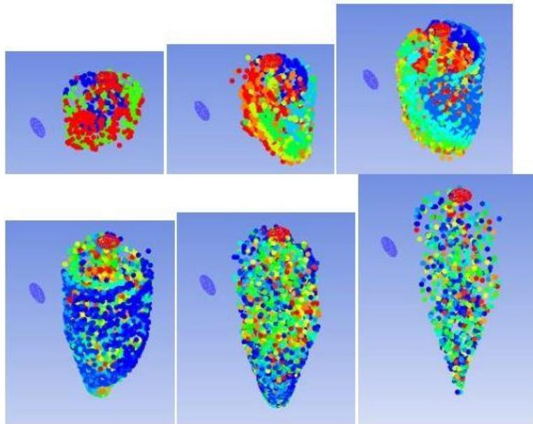
Fig. 4 Particle distribution at different time (Ansys fluent simulation)
