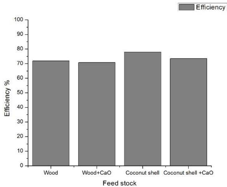
Fig. 5 Efficiency of cyclone for different feedstock (practically)
