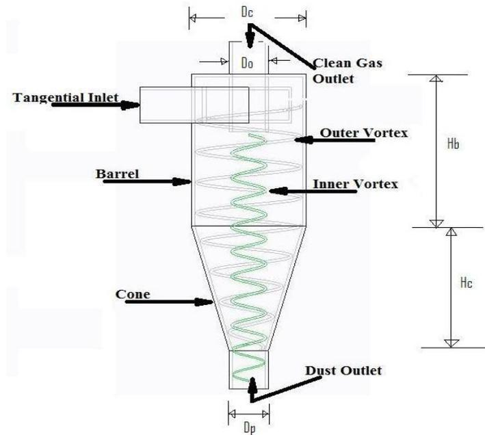
Fig. 2 Schematic of cyclone separator
