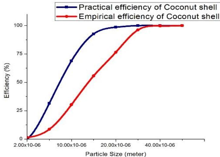
Fig. 9 Efficiency comparisons experimentally v/s Empirical model for feed stock Coconut shell
