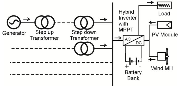
Fig. 1 One line diagram of HPS with power flow of grid
