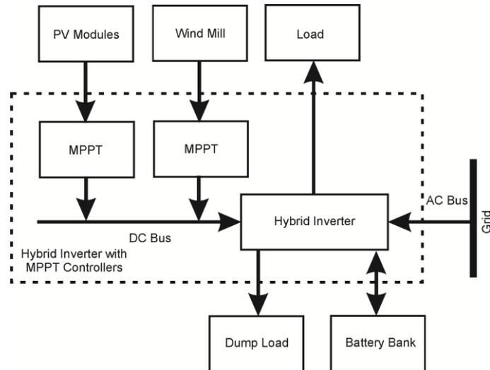
Fig. 2 Configuration of the proposed hybrid power system
