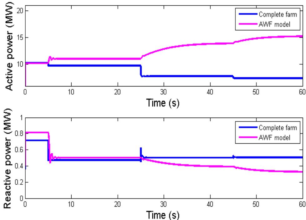
Fig. 7 Comparison at PCC without controller
