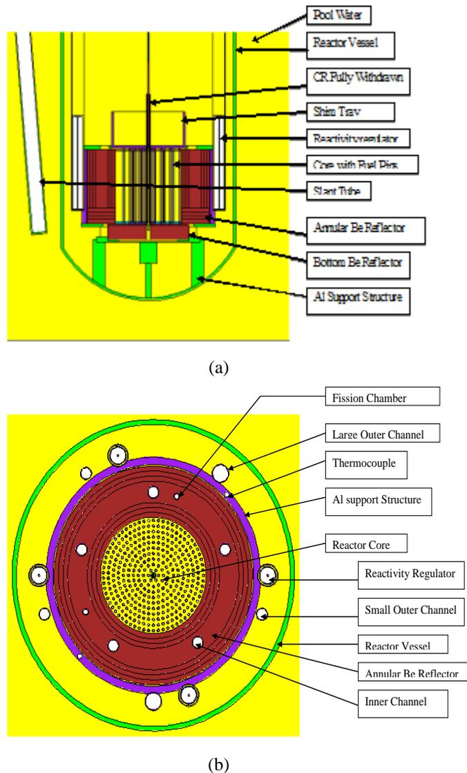
Fig. 1 MCNP Axial and Radial view of NIRR-1
