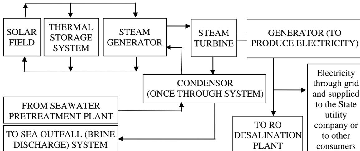
Fig. 2 Block diagram for solar power plant in Copper industry
