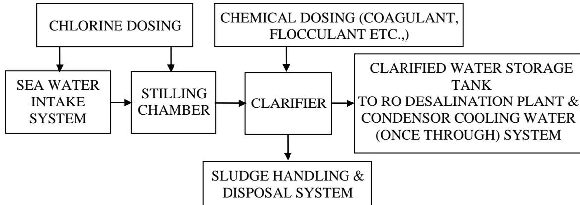
Fig. 1 Block diagram for seawater pretreatment plant in Copper industry.
