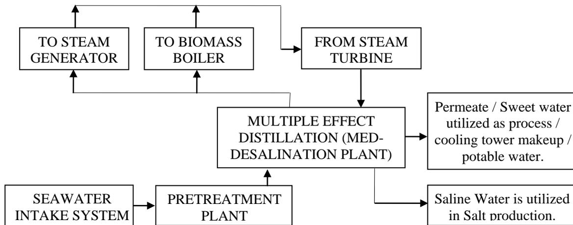
Fig. 5 Block diagram (modified) for desalination plant in Copper industry
