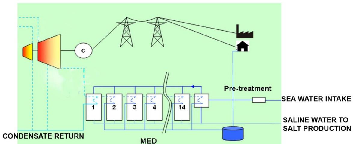
Fig. 6 Flow diagram (modified) showing MED desalination plant in Copper industry
