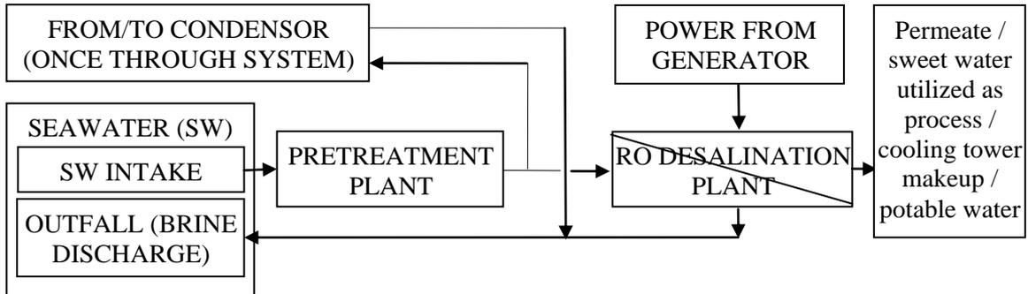
Fig. 3 Block diagram for RO Desalination plant in Copper industry
