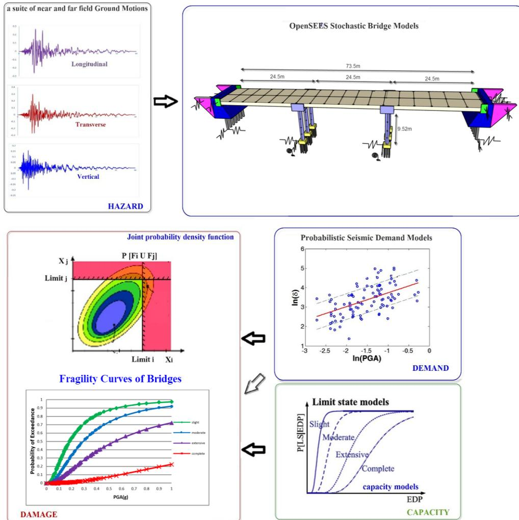
Fig. 9 Schematic of the probabilistic seismic assessment framework
