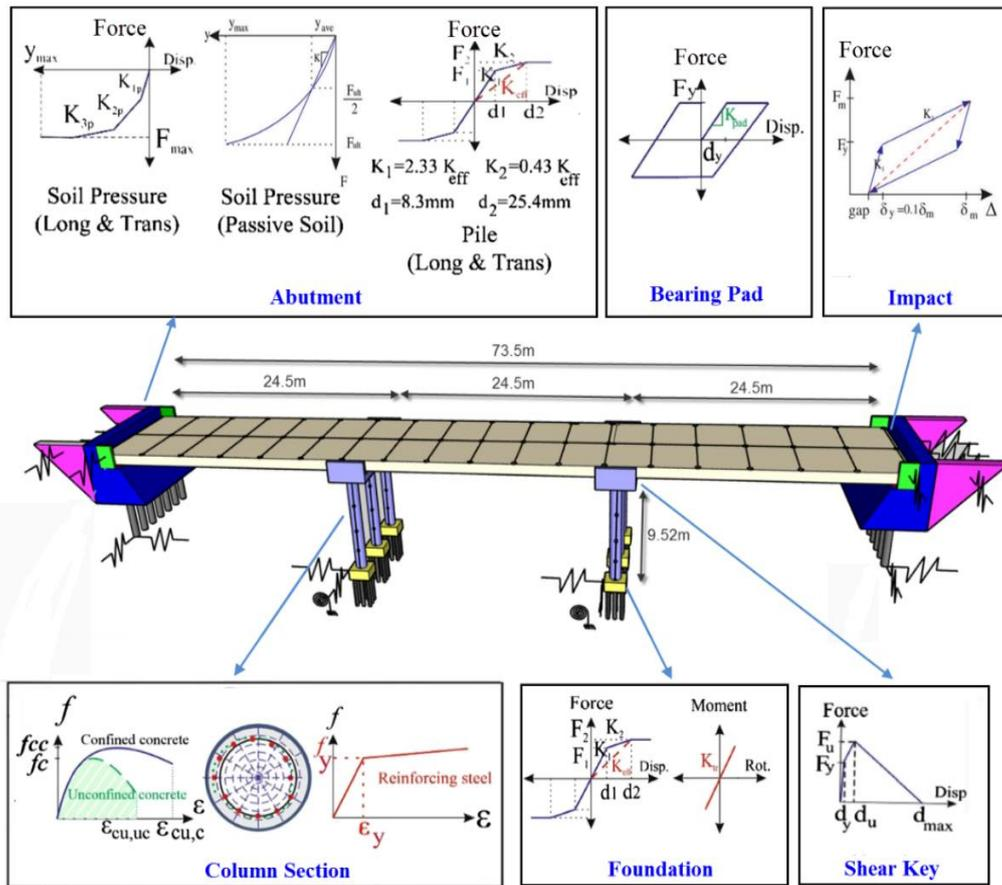
Fig. 7 Analytical model of the bridge and components with nonlinear behaviors
