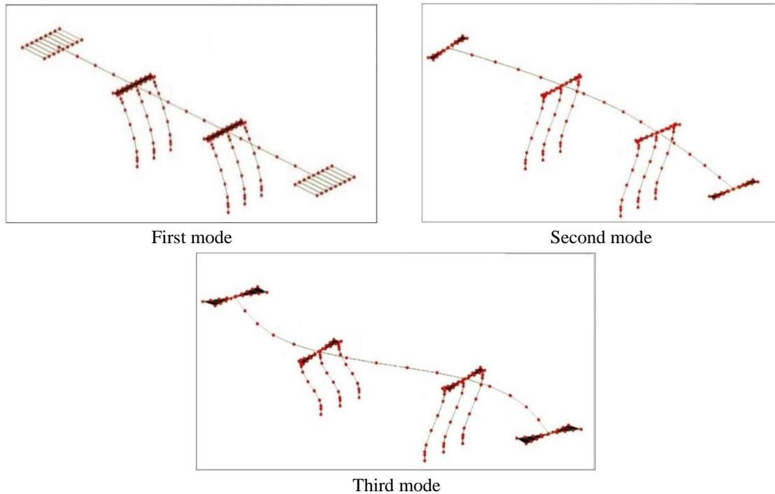
Fig. 8 The first three modes of the bridge
