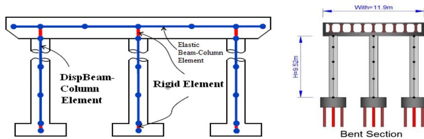
Fig. 6 Modeling of the deck, columns, and column caps in *OpenSEES* platform
