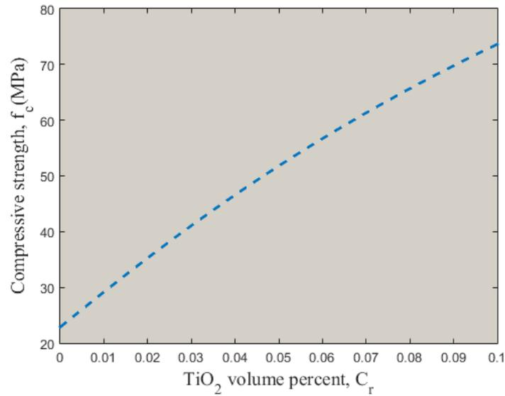
Fig. 2 The effect of TiO<sub>2</sub> nanoparticles on the compressive strength of the concrete
