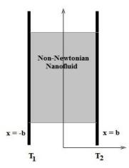
Fig. 1 Nanofluid flow between two vertical flat plates
