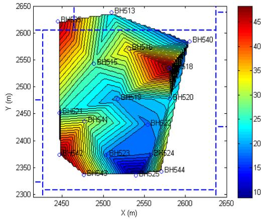
Fig. 6 SPT-N Contour using linear interpolation (at depth=20 m)
