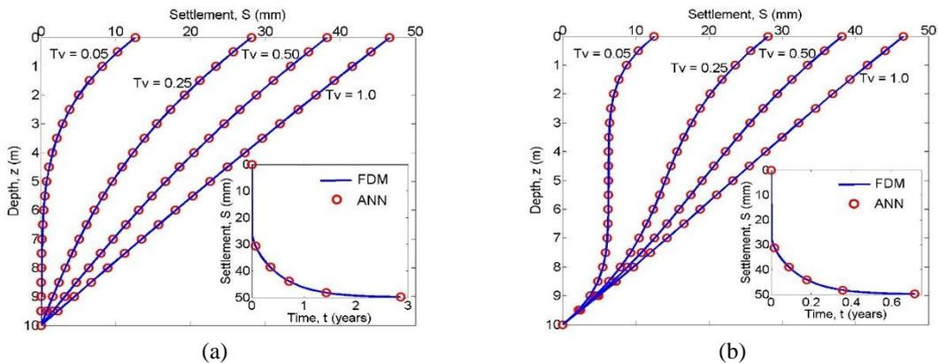
Fig. 12 Comparison of predicted settlements between FDM and ANN
