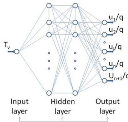
Fig. 9 Typical architecture of the ANN model for 1D consolidation prediction
