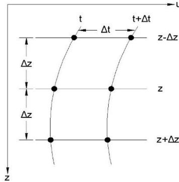
Fig. 8 Finite difference nodes in the numerical solution of the 1D consolidation equation
