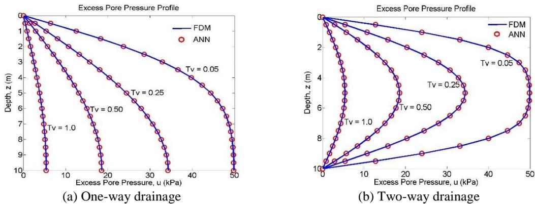
Fig. 11 Comparison of predicted excess pore pressure profiles between FDM and ANN
