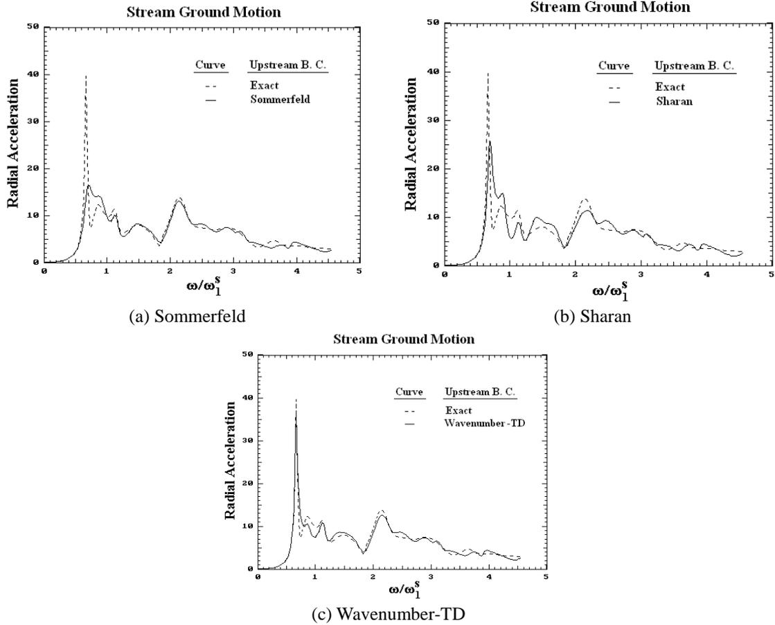
Fig. 4 Radial acceleration at dam crest due to stream ground motion for different absorbing boundary condition alternatives ( $L/H=1, \alpha=1$ )
