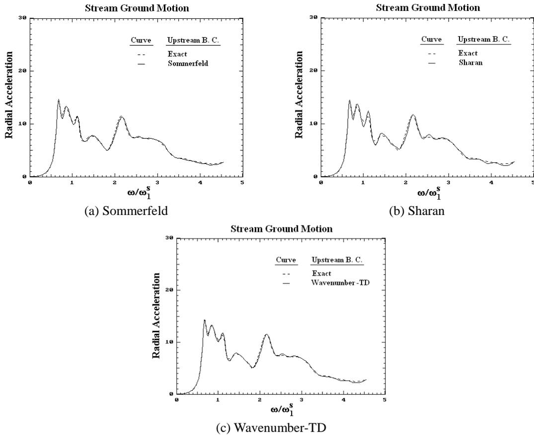
Fig. 8 Radial acceleration at dam crest due to stream ground motion for different absorbing boundary condition alternatives ( $L/H=3$ ,  $\alpha=0.85$ )
