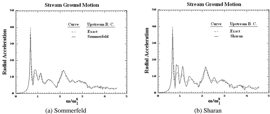
Fig. 5 Radial acceleration at dam crest due to stream ground motion for different absorbing boundary condition alternatives ( $L/H=3, \alpha=1$ )
