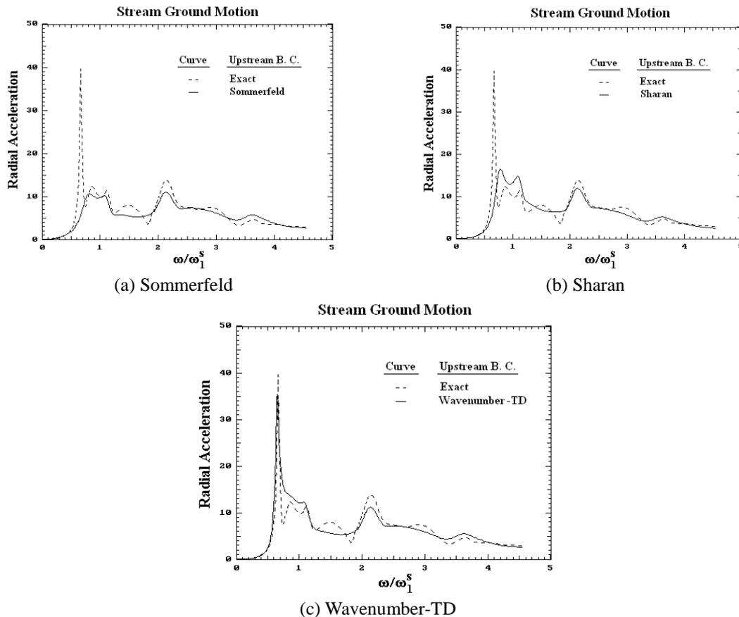
Fig. 3 Radial acceleration at dam crest due to stream ground motion for different absorbing boundary condition alternatives ( $L/H=0.2$ ,  $\alpha=1$ )
