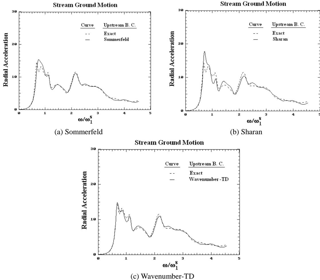
Fig. 7 Radial acceleration at dam crest due to stream ground motion for different absorbing boundary condition alternatives ( $L/H=1$ ,  $\alpha=0.85$ )
