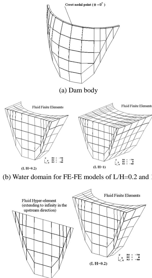
Fig. 2 Discretization of dam-reservoir system
