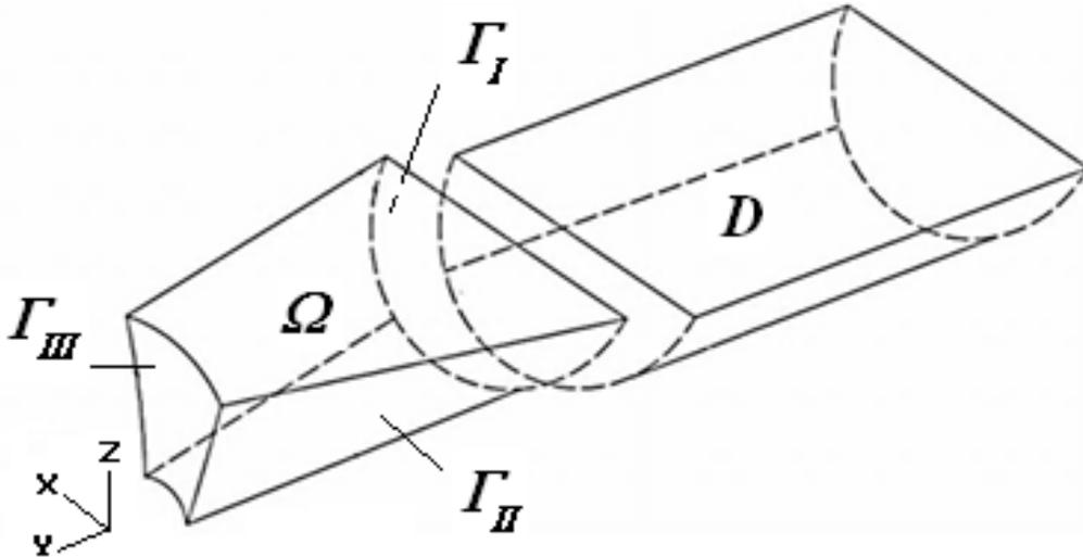
Fig. 1 Schematic view of a typical reservoir (i.e., water domain). The near-field reservoir domain  $\Omega$ , the truncation boundary  $\Gamma_I$  and the far-field region  $D$  (excluded in the FE-FE type of analysis)
