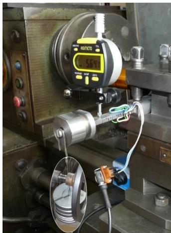
Fig. 5 Experimental determination of the dependence  $w(\xi) = f(T)$
