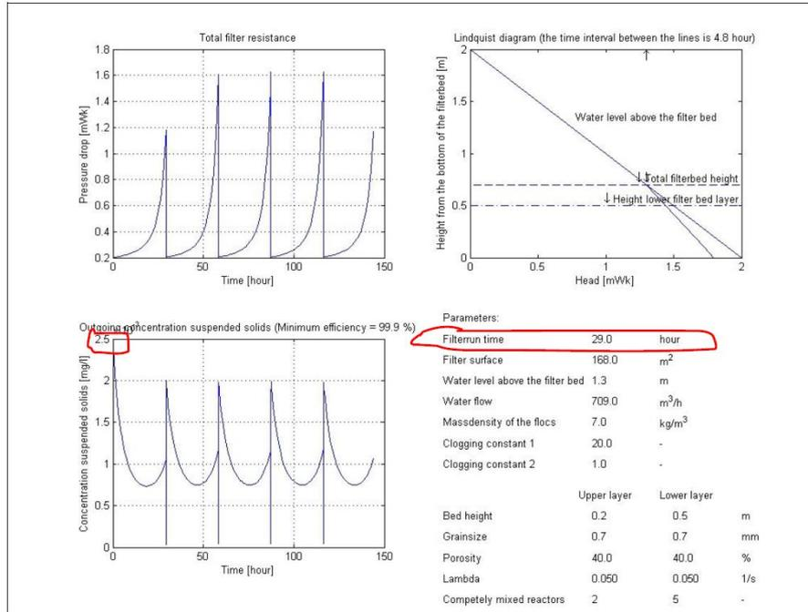
Fig. 8 Output results of simulation for input turbidity 2,5NTU – filter run time 29h (Jusic 2011)
