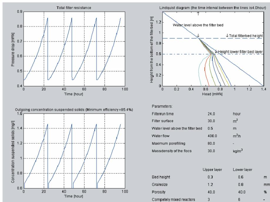
Fig. 5 Graphical output of simulation of (dual media) filtration (Rietveld 2005)
