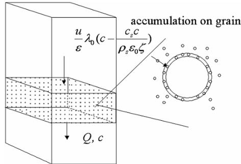
Fig. 3 Schematic impression of rapid filtration (Rietveld 2005)
