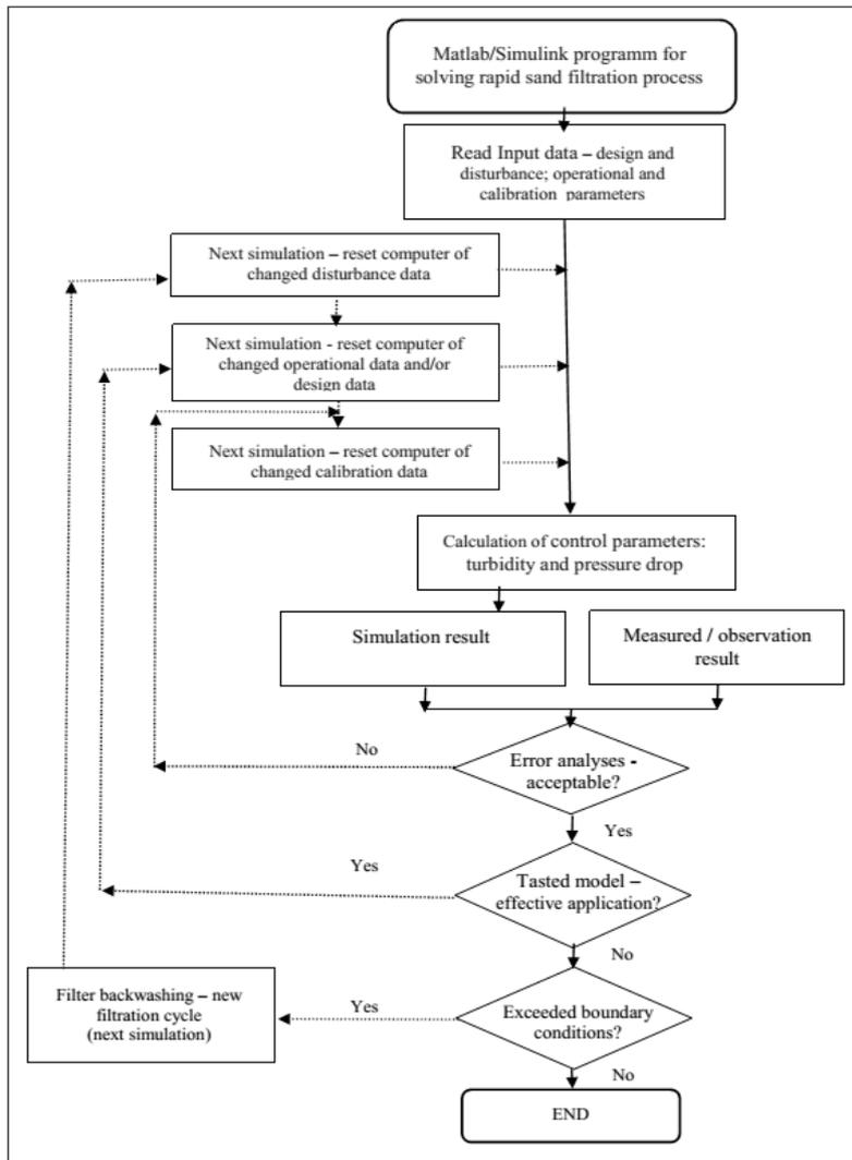
Fig. 4 Algorithm for rapid sand filtration process through Stimela model (Jusic 2011)
