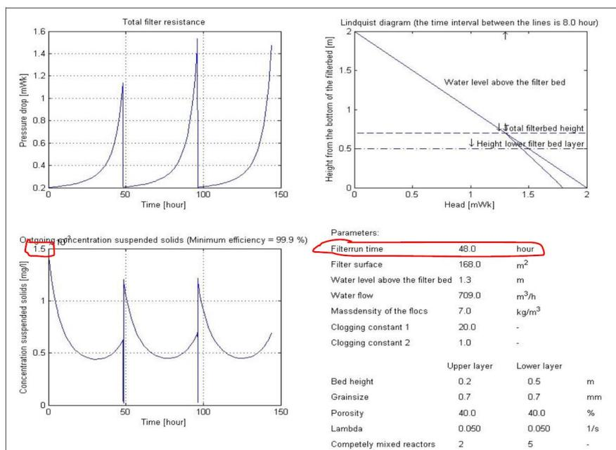
Fig. 11 Output result of simulation for input turbidity 1,5 NTU – filter run time 48h (Jusic 2011)
