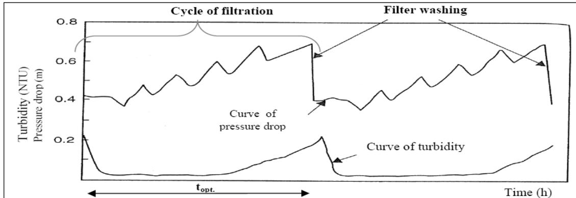
Fig. 1 A typical diagram of the dependence of filtered water turbidity and pressure losses in time – two cycles of filtration (Jusic 2012)
