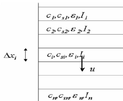
Fig. 2 Schematic representation of filter bed (Van Schagen 2009)
