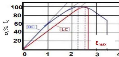
Fig. 1 Stress-strain dependence in compression test for DC and LC with the same strength (Szydlowski and Mieszczak 2017)
