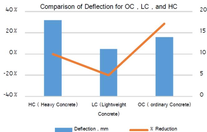
Fig. 10 Deflections for slabs (OC, LC, and HC)
