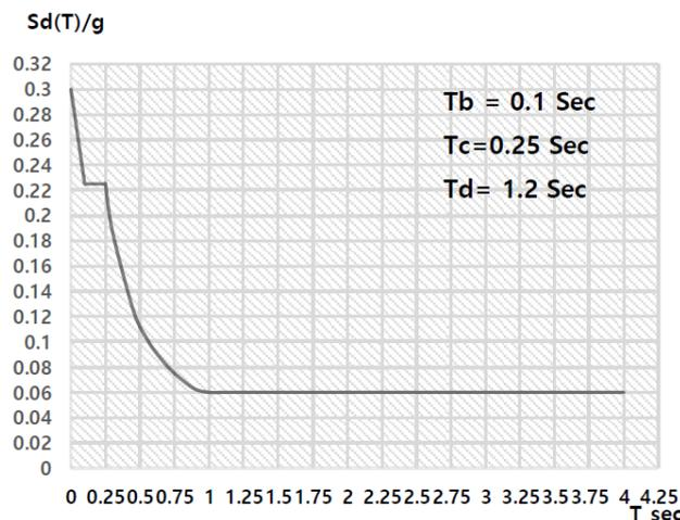
Fig. 3 Response spectrum curve (RES)
