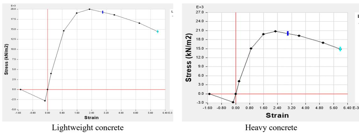
Fig. 2 Stress-strain curve for (LC, OC, and HC)
