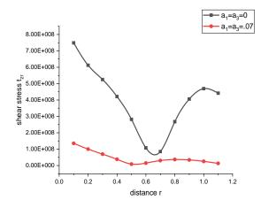
Fig. 8 Variation of shear stress  $t_{zr}$  with the distance r
