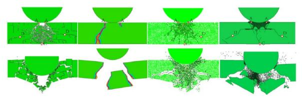
Fig. 7 Evolution of crack pattern for different calculation methods (from left to right FEM, XFEM, DEM and FEM/DEM respectively) (Wang *et al.* 2017)
