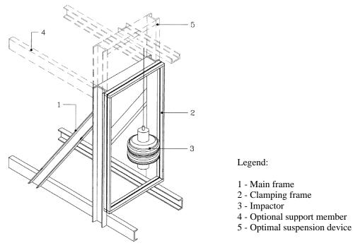
Fig. 2 Test setup for soft body impact according to HR EN 12600:2006 (EN 12600:2002)
