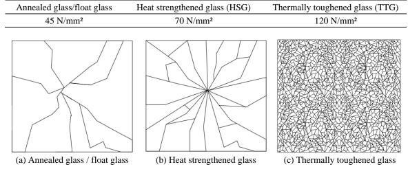
Fig. 1 Breakage pattern for each type of glass
