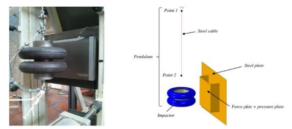
Fig. 5 Test setup with pendulum and pressure plate, simulation of pendulum test (Pelfrene et al. (2016))
