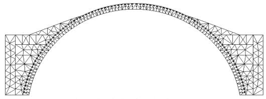
Fig. 16 Discretisation of the Old Bridge model
