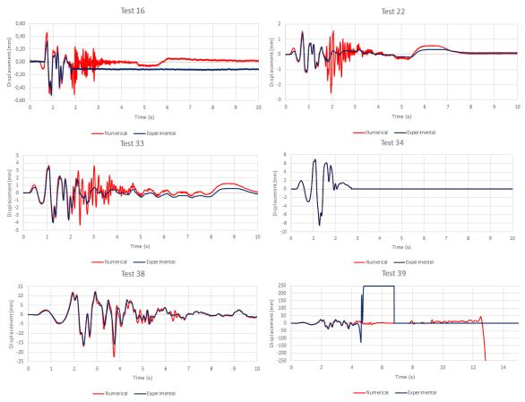
Fig. 18 Comparison of the time histories of the horizontal displacements at the top of the arch
