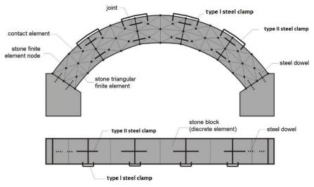
Fig. 15 Discretisation of a stone arch with installed clamps and dowels [11]
