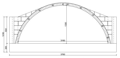
Fig. 5 Geometry of the model of the Old Bridge - front view (cm)
