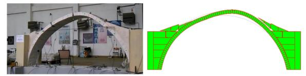
Fig. 20 Mode shapes and failure mechanism for Test\_39-initial cracks
