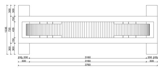
Fig. 6 Geometry of the model of the Old Bridge - top view (cm)
