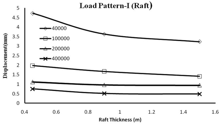
Fig. 4 Variations in maximum deflection for raft foundation (LP-I)
