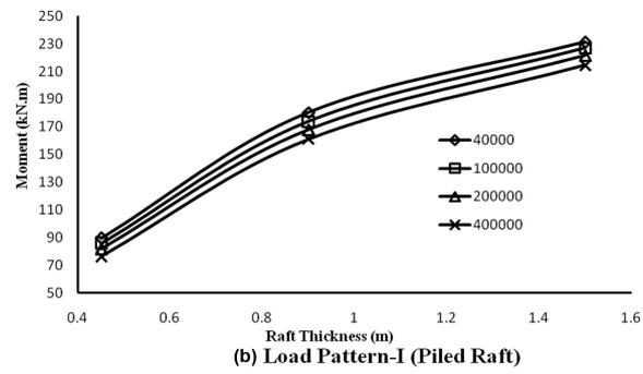
Fig. 10 Comparison of maximum moment for load pattern-I
