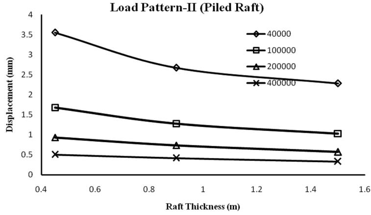
Fig. 7 Variations in maximum deflection for piled-raft foundation (LP-II)
