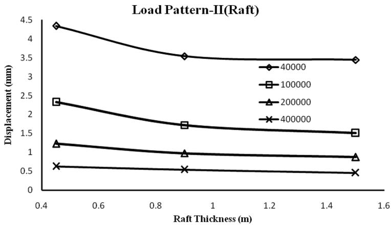
Fig. 6 Variations in maximum deflection for raft foundation (LP-II)
