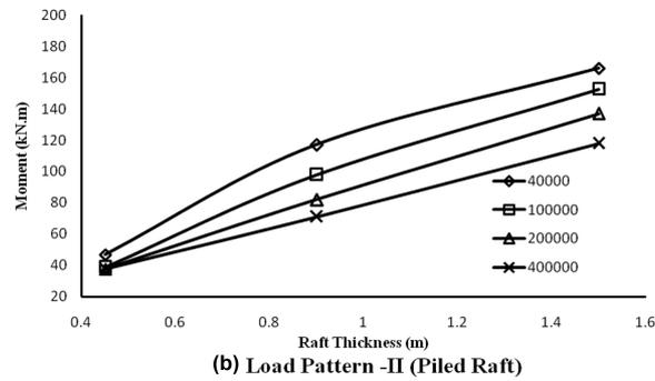
Fig. 11 Comparison of maximum moment for load pattern-II
