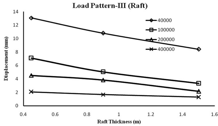
Fig. 8 Variations in maximum deflection for raft foundation (LP-III)
