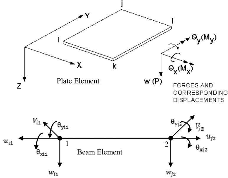
Fig. 2 Rectangular plate element and Beam element
