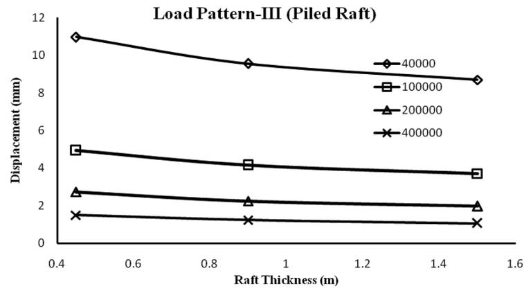
Fig. 9 Variations in maximum deflection for piled-raft foundation (LP-III)
