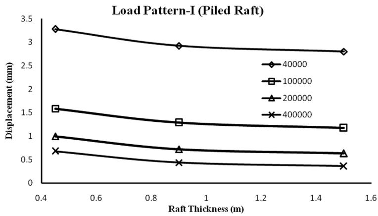
Fig. 5 Variations in maximum deflection for piled-raft foundation (LP-I)
