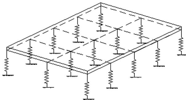
Fig. 1 Structural idealization of raft and supporting soil
