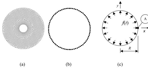
Fig. 3 Circular cavity: (a) FEM mesh, (b) BEM mesh and (c) geometry and boundary conditions
