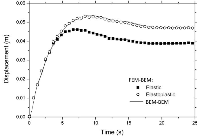
Fig. 4 Horizontal displacements at point *A* considering elastic and elastoplastic behaviour
