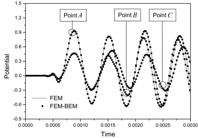
Fig. 2 Time history results at points *A*, *B* and *C* for the fluid-fluid interaction analysis
