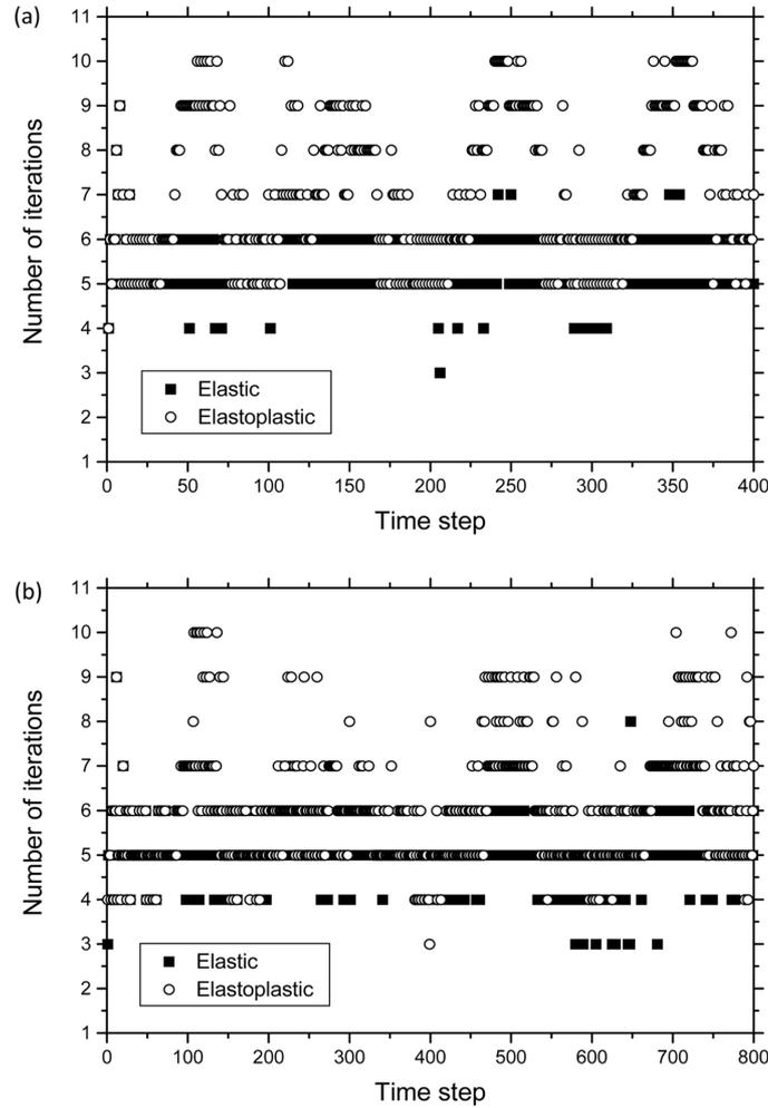
Fig. 9 Number of iterations per time step considering optimal relaxation parameters: (a) case 1 and (b) case 2
