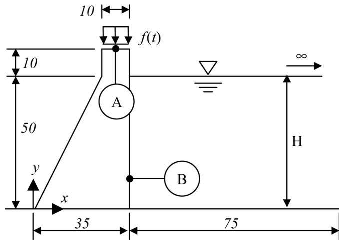
Fig. 7 Dam with a semi-infinite storage-lake: sketch of the model
