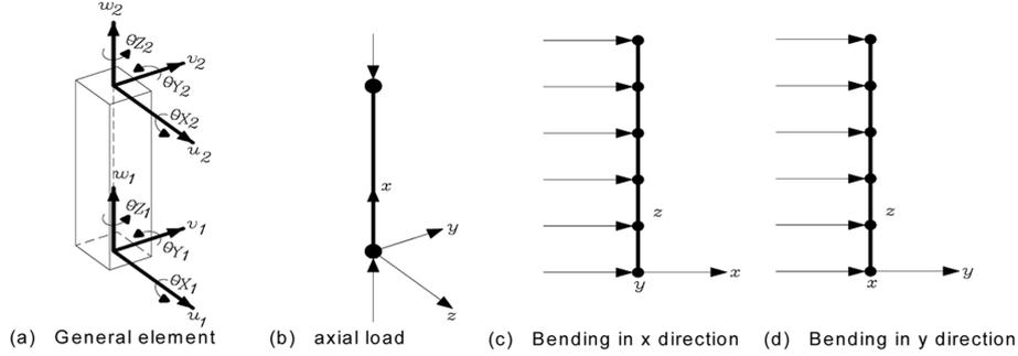
Fig. 1 General beam-column element Desai *et al.* (1981)
