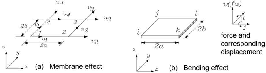
Fig. 2 A schematic of general plate element Zienkiewicz (1977)
