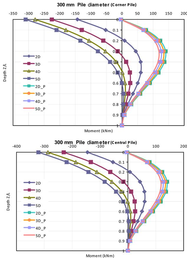
Fig. 8 Variation of moment along depth of pile (Group of three piles)
