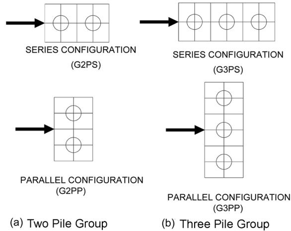
Fig. 3 Different configurations considered in the study
