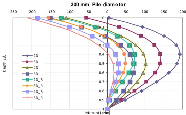
(b) Comparison of moments in front and rear pile (series configuration)
