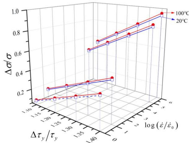
Fig. 9 The effect of interfacial shear strength on tensile strength
