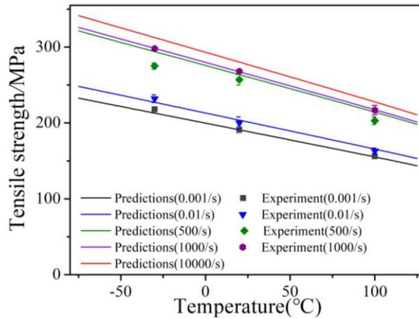
Fig. 2 The change of tensile strength with temperature at different strain rates
