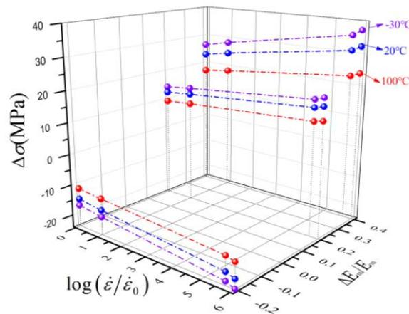
Fig. 8 The effect of Young's modulus of matrix on tensile strength
