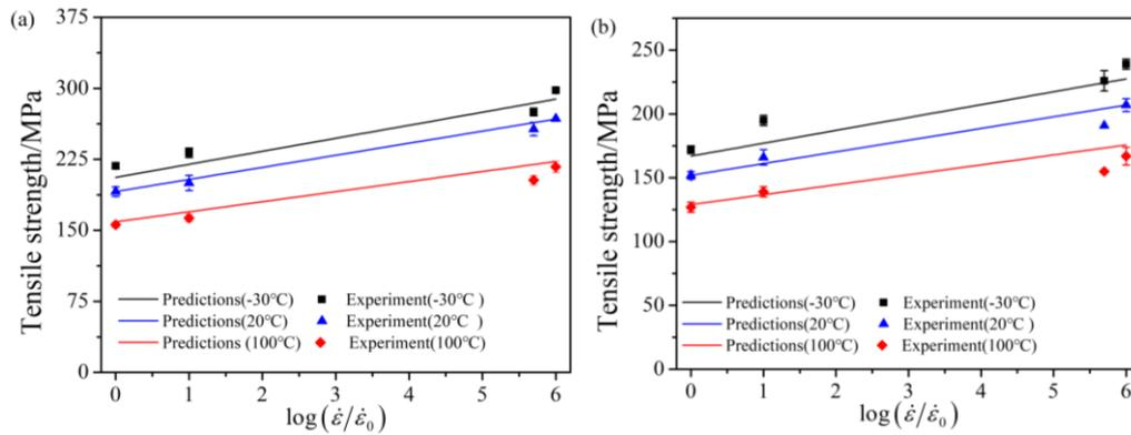
Fig. 1 Temperature and strain rate dependent tensile strength of short (a) carbon fiber and (b) glass fiber reinforced PEEK composites (The experimental data are quoted from Chen (2019))
