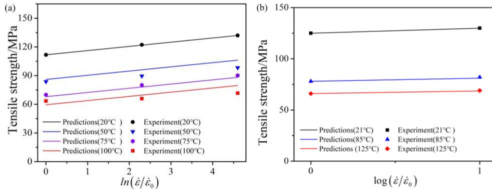
Fig. 3 Temperature and strain rate dependent tensile strength of short glass fiber/PA6 composites: (a) 33% vol fiber (The experimental data are quoted from Wang *et al.* (2002)) (b) 35% vol fiber (The experimental data are quoted from Mortazavian and Fatemi (2017))
