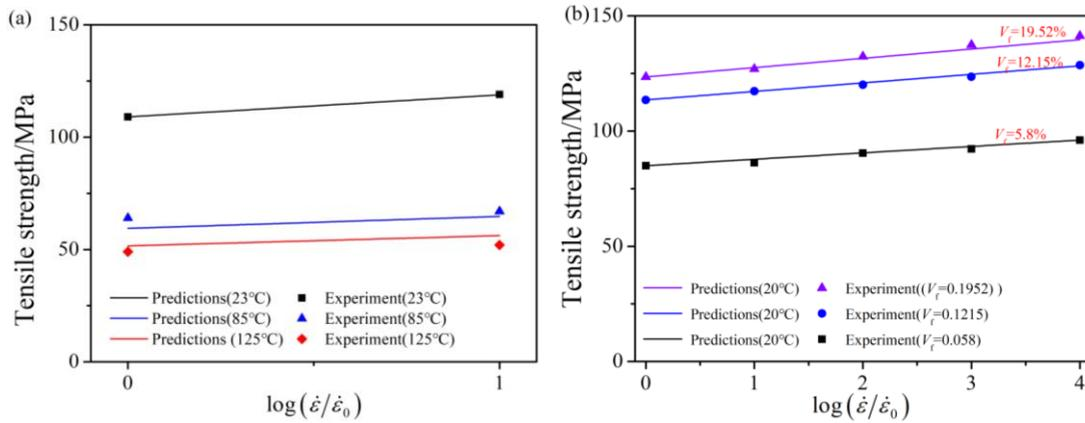
Fig. 4 Tensile strength of PBT composites (a) At different temperatures and strain rates (The experimental data are quoted from Mortazavian and Fatemi (2017)) (b) Under different fiber content (The experimental data are quoted from Hashemi (2011))
