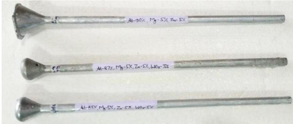
Fig. 1 Developed samples from stir casting
