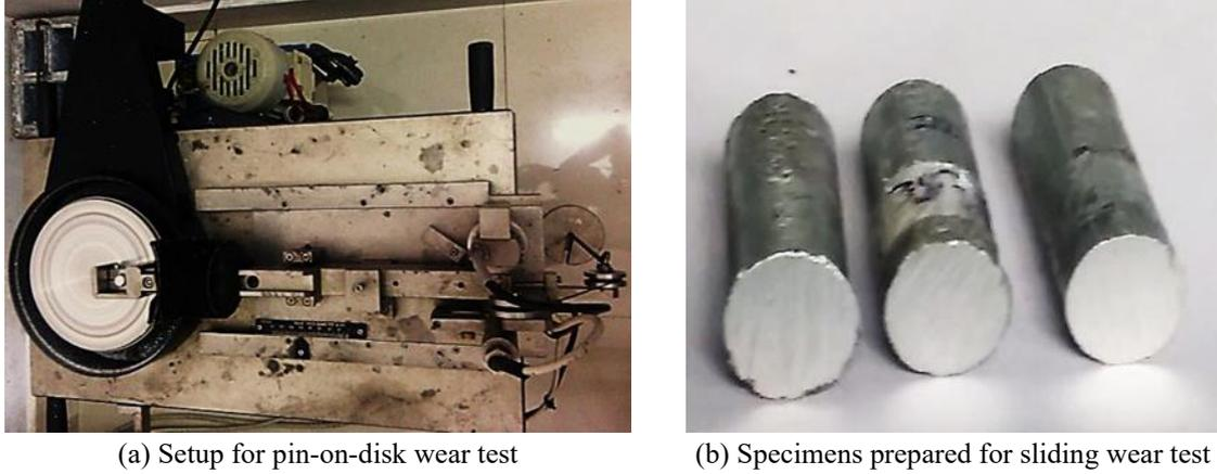
(a) Setup for pin-on-disk wear test
