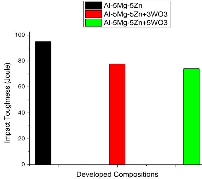
Fig. 4 Impact toughness of the developed compositions
