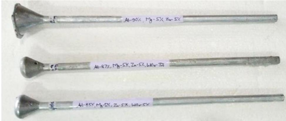
Fig. 1 Developed samples from stir casting
