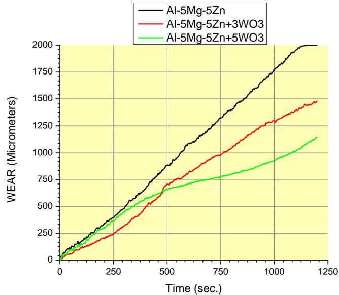
Fig. 5 Dry sliding wear graph of the developed compositions
