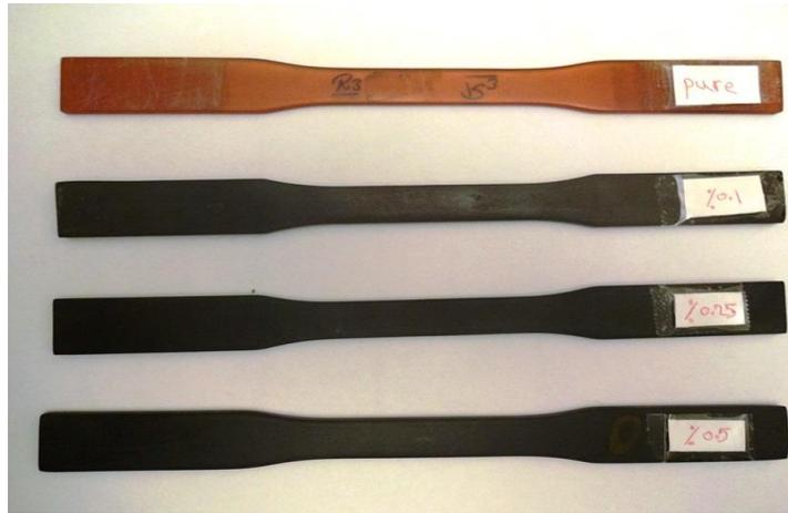
Fig. 1 Pure epoxy and GNP/epoxy samples fabricated for tensile tests
