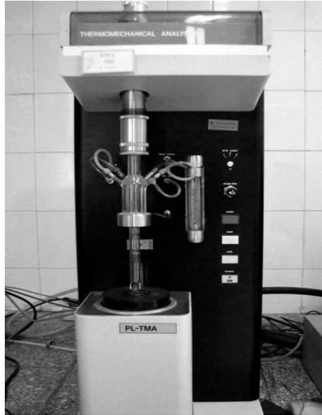
Fig. 3 PL-TMA CTE measurement device (Iran Polymer and Petrochemical Institute)
