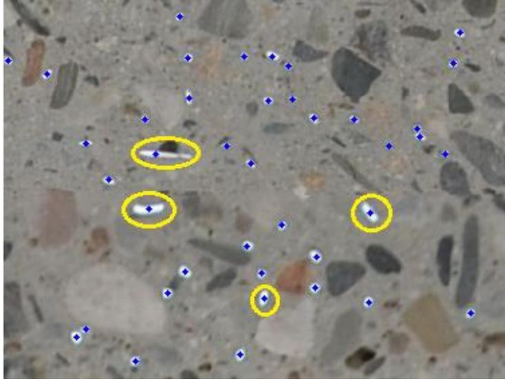
Fig. 5 Detail showing one part of analyzed SFRC cross-section. Fibers highlighted by yellow ellipses are the fibers that were cut askew (i.e. the cut plane was not perpendicular to the longitudinal axis of the fiber). Special inbuilt subroutine of ASEF guarantees that the whole cross-section will be treated as one fiber
