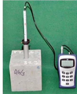
(b) Depth magnetic probe in SFRC sample
