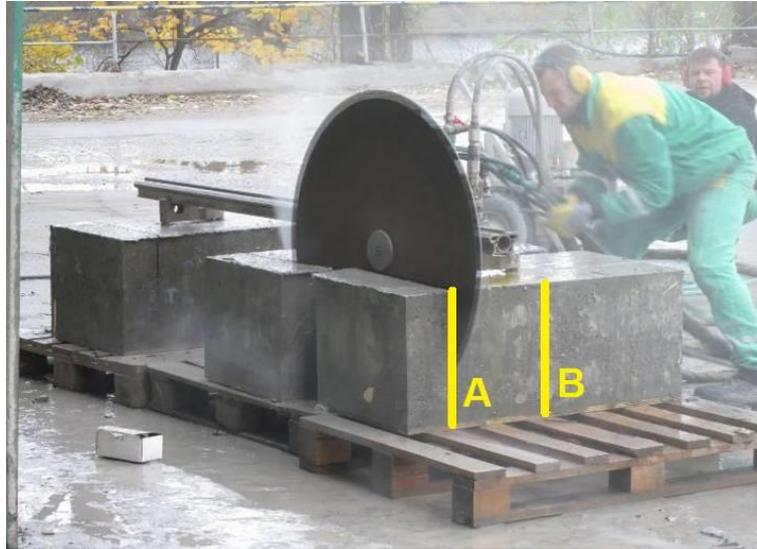
Fig. 11 Sawing of large scale SFRC specimens
