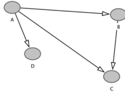
Fig. 5 Illustration of a DAG [corresponding SEMs are,  $D := f_1(A)$ ,  $B := f_2(A)$ ,  $C := f_3(A, B)$ . Note that error terms are assumed independent and are not explicitly shown in the figure. Also,  $:=$  implies a causal statement]
