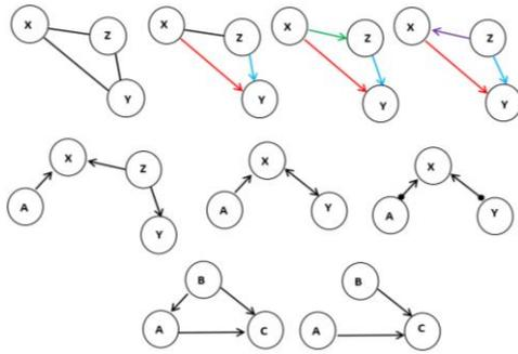
Fig. 7 Graphs [Note from the top row and going right: graph (skeleton), CPDAG, DAG Markov equivalent 1, DAG Markov equivalent 2. Middle row left and going right: Assumed true DAG, MAG, and PAG. Bottom row: DAG, DAG with an intervention on A (i.e.,  $do(A=a)$ )]
