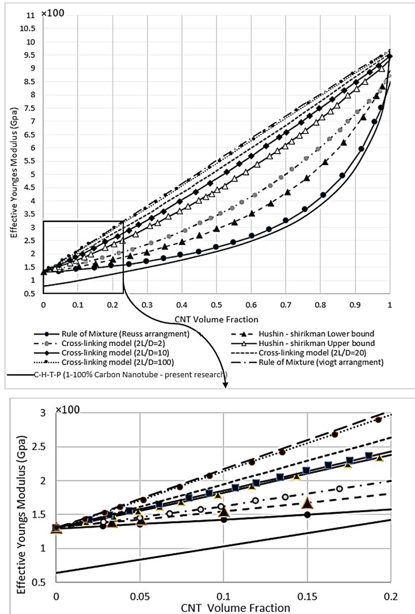
Fig. 5 Compression of elasticity modulus in the introduced bone scaffold with the bone scaffolds presented by (PourAkbar Saffar *et al.* 2010), in terms of volume fraction of carbon nanotubes
