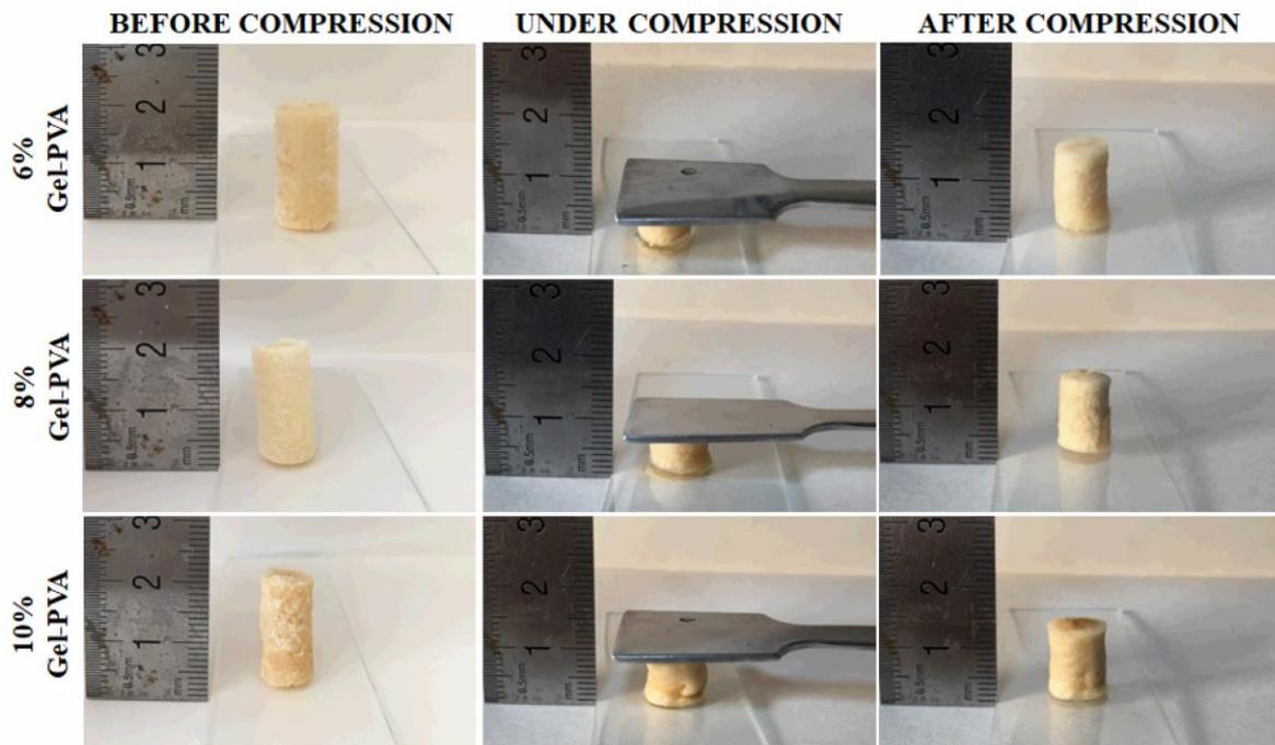
Fig. 3 Images of Gel-PVA cryogels (before, under and after compression)
