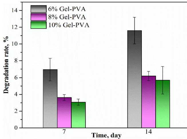
Fig. 5 Degradation profile of Gel-PVA cryogels
