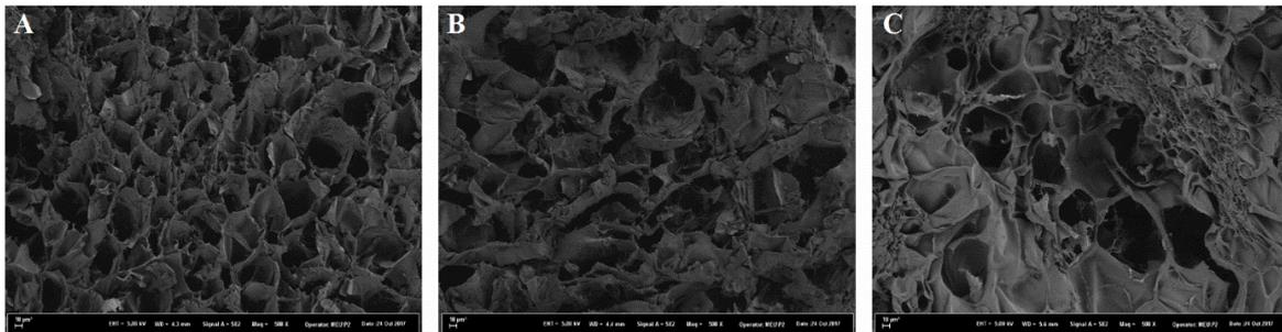
Fig. 2 SEM images of cryogels (A: 6% Gel-PVA, B: 8% Gel-PVA, C: 10% Gel-PVA at magnification of 500x)
