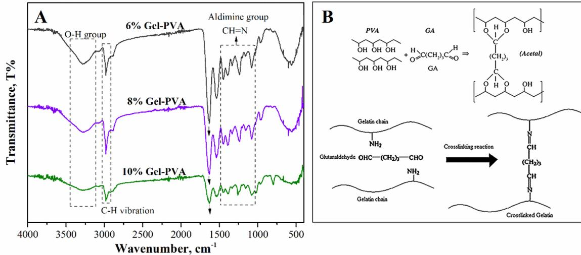
Fig. 1 A) FTIR spectra of cryogels B) Reaction mechanism of PVA-Glutaraldehyde and Gelatin-Glutaraldehyde
