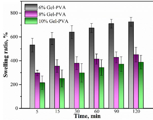
Fig. 4 Swelling profile of Gel-PVA cryogels
