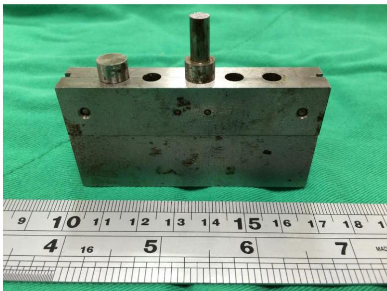
Fig. 1 Photo of the mold used to fabricate the 5 mm beads
