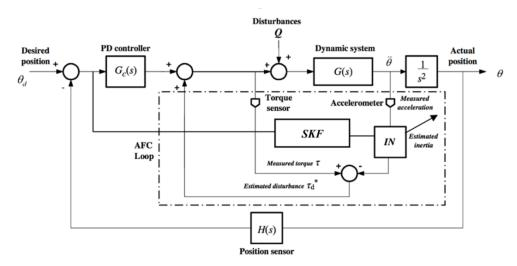
Fig. 1 The PD with SKF based AFC scheme for the control of the upper limb exoskeleton
