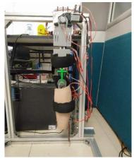
Fig. 3 The upper limb exoskeleton system
