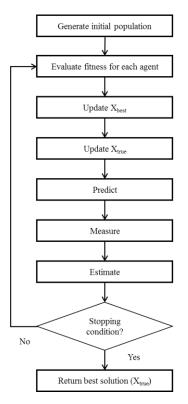
Fig. 2 The SKF algorithm
