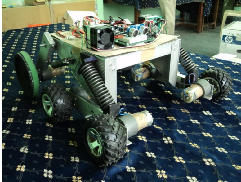
Fig. 1 Photograph showing prototype of the developed all-terrain robot
