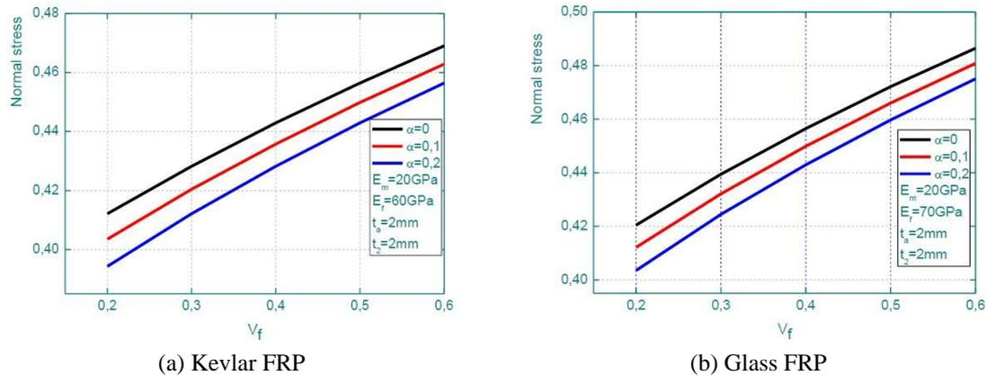
Fig. 10 Porosity effect as function of fibers volume fraction on normal stress of RC beam strengthened with Kevlar and Glass FRP plate
