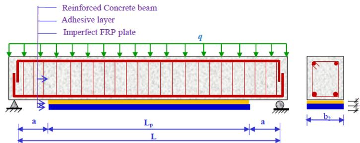
Fig. 2 Simply supported RC beam strengthened with bonded imperfect FRP plate
