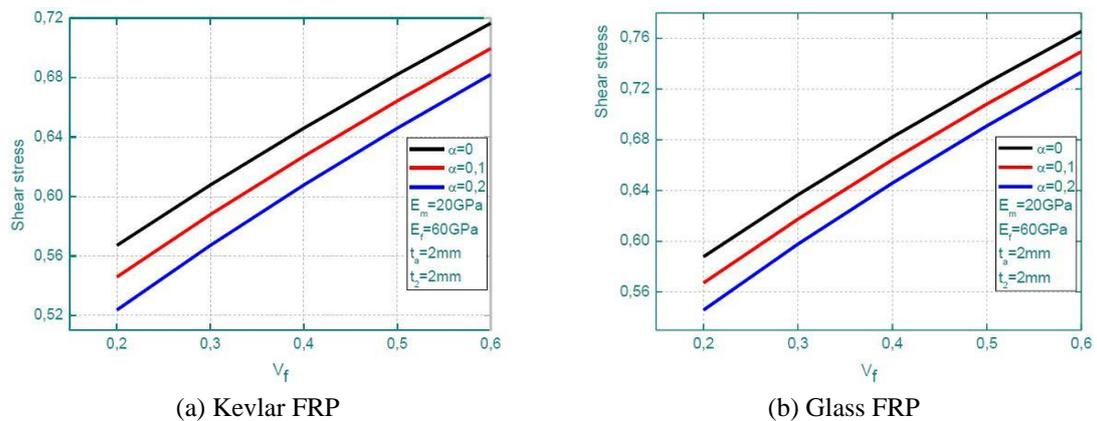
Fig. 11 Porosity effect as function of fibers volume fraction on shear stress of RC beam strengthened with Kevlar and Glass FRP plate
