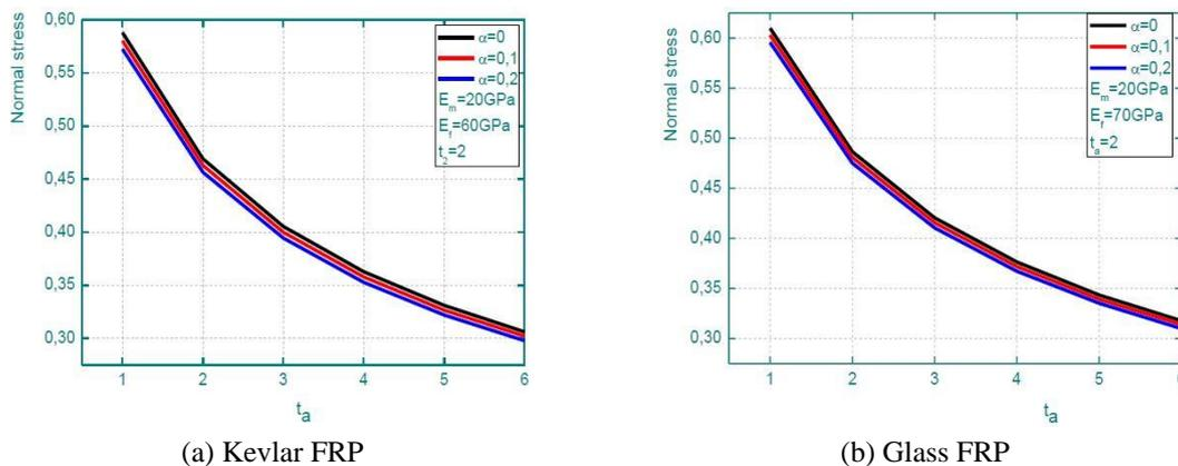
Fig. 6 Porosity effect as function of adhesive thickness on normal stress of RC beam strengthened with Kevlar and Glass FRP plate
