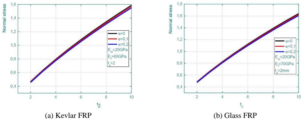
Fig. 4 Porosity effect as function of plate thickness on normal stress of RC beam strengthened with Kevlar and Glass FRP plate
