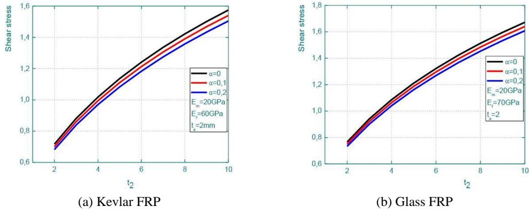
Fig. 5 Porosity effect as function of plate thickness on shear stress of RC beam strengthened with Kevlar and Glass FRP plate
