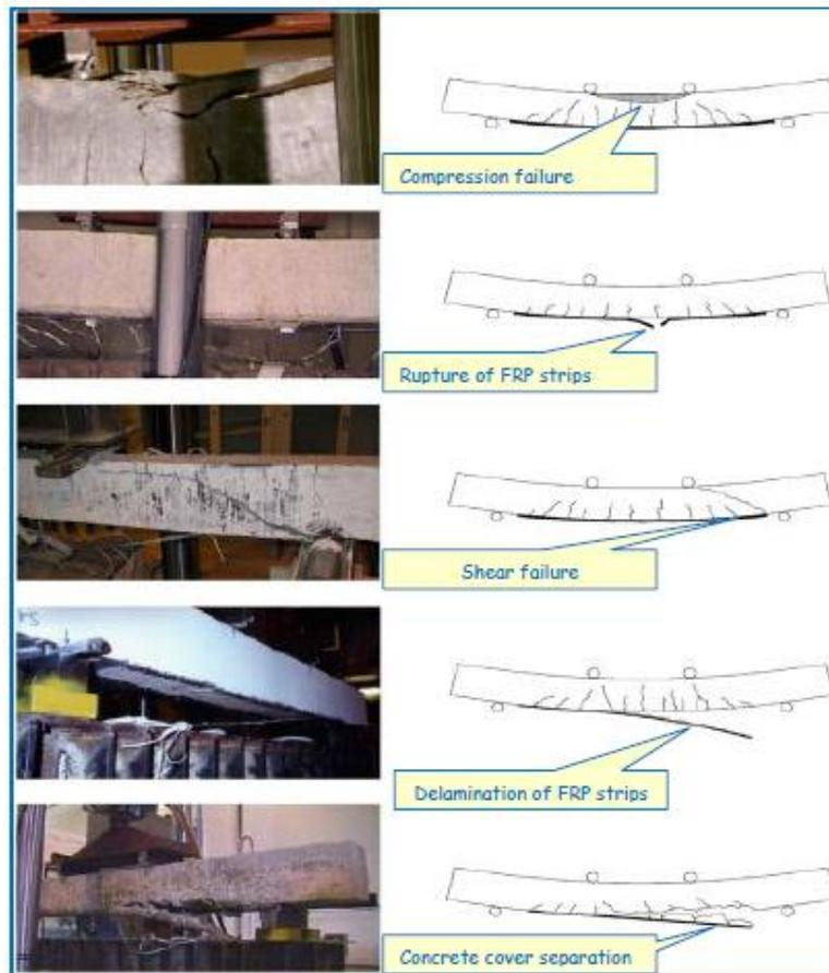
Fig. 1 Failure modes of FRP strengthened RC beams
