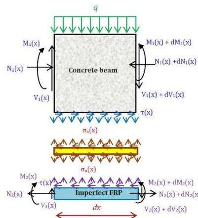
Fig. 3 Forces in differential element of the plated beam
