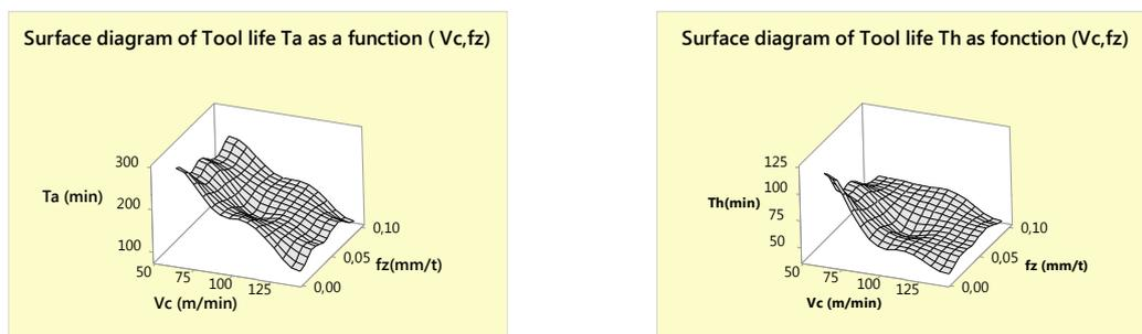
Fig. 4 Surface diagram of tool life  $Ta$  and  $Th$  versus cutting conditions
