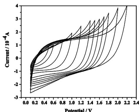
Fig. 4 Cyclic voltammograms obtained by varying the potential window of cycling at the scan rate of 10 mV/s at room temperature
