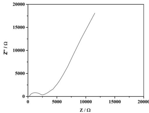
Fig. 1 One of the resulted nyquist plots of an EDLC at room temperature
