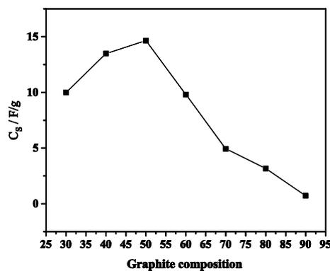
Fig. 3 Variation of single electrode specific capacity ( $C_s$ ) with the amount of graphite in the electrode at room temperature
