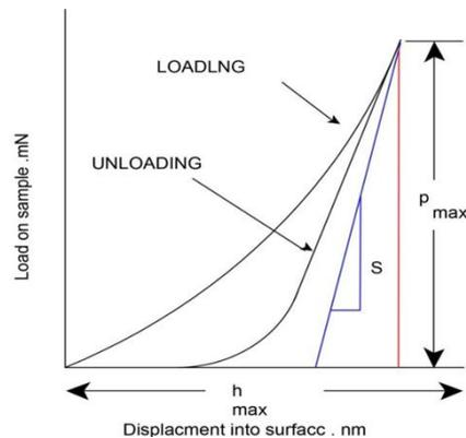
Fig. 3 Adaptation curves (loading and unloading) from a nano-indentation test
