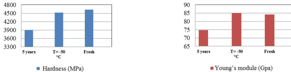
(a) Hardness of top neck mollusks shell samples in different situations and directions (b) The young's modulus of top neck mollusk shell samples in different situations and directions
