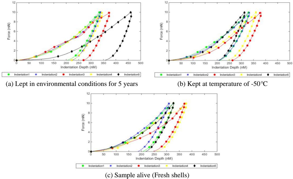
Fig. 4 Force-Indentation depth diagram of top neck mollusks shell samples
