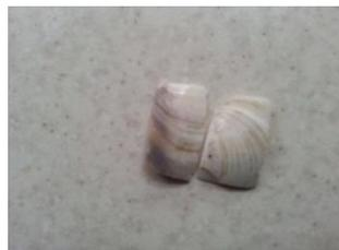
(b) Sample preparation for nano-indentation test
