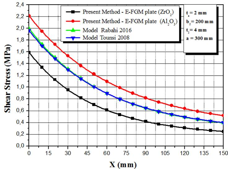
Fig. 5 Comparison of shear interfacial stress in RC beam bonded with prestressed E-FGM plate  $P_0=0$
