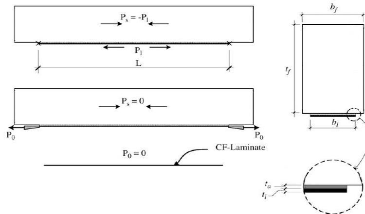
Fig. 1 A reinforced concrete beam strengthened with bonded prestressed E-FGM plate
