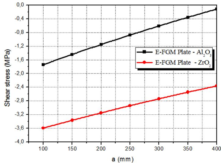
Fig. 9 Effect of length of unstrengthened region on interfacial stress in prestressed E-FGM strengthened RC beam
