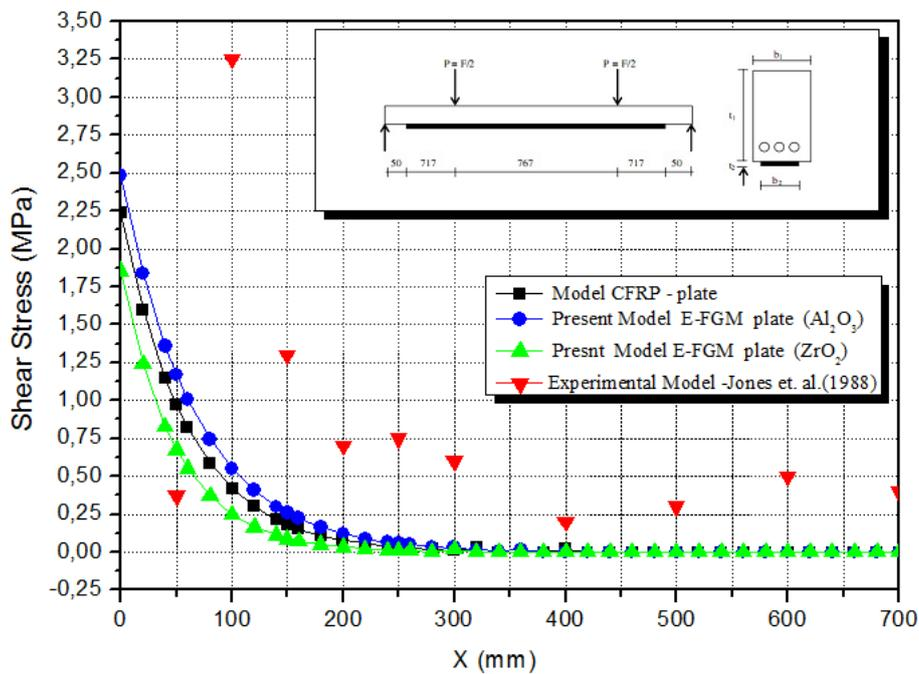
Fig. 4 Comparison of interfacial shear of the GFRP and E-FGM plated RC beam with the experimental results
