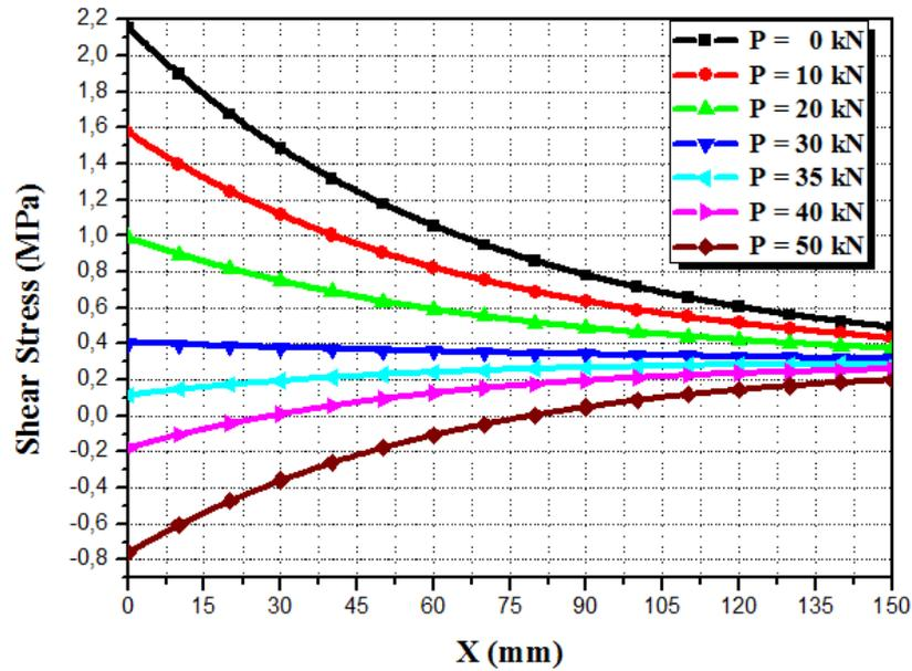
Fig. 6 Adhesive shear stress along the bond line for prestressed E-FGM ( $\text{Al}_2\text{O}_3$ ) strengthened
