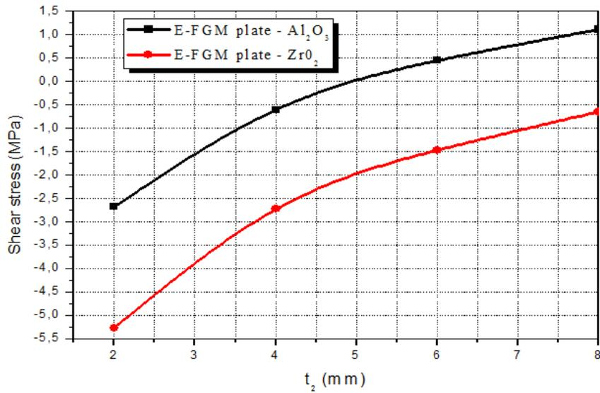
Fig. 7 Effect of plate thickness on interfacial shear stress in prestressed E-FGM strengthened RC beam
