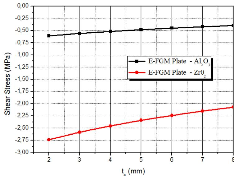
Fig. 8 Effect of adhesive layer thickness on interfacial shear stress in prestressed E-FGM strengthened RC beam
