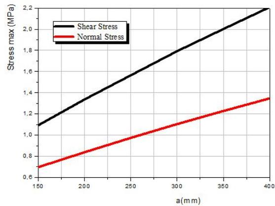
Fig. 4 Influence of length of unstrengthened region on edge stresses for RC beam with a bonded sandwich FGM plate
