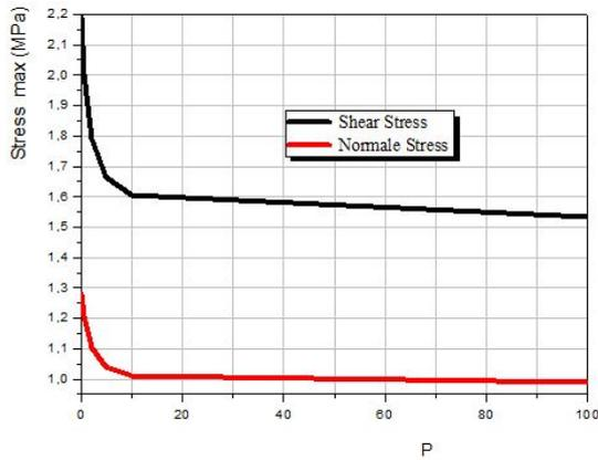
Fig. 3 Effect of degree of homogeneity on interfacial stresses in sandwich FGM plate strengthened RC beam
