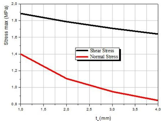
Fig. 6 Effect of adhesive layer thickness on edge shear stresses in sandwich FGM plate strengthened RC beam
