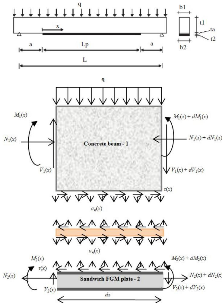
Fig. 1 Simply supported RC beam strengthened with sandwich FGM plate
