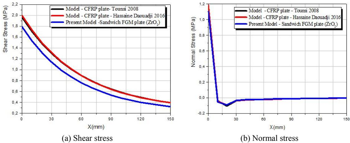
Fig. 2 Comparison of interfacial shear and normal stress for sandwich FGM plate RC beam with the analytical results
