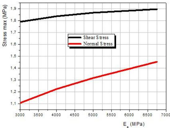
Fig. 5 Effect of adhesive moduli on interfacial stresses in sandwich FGM plate strengthened RC beam
