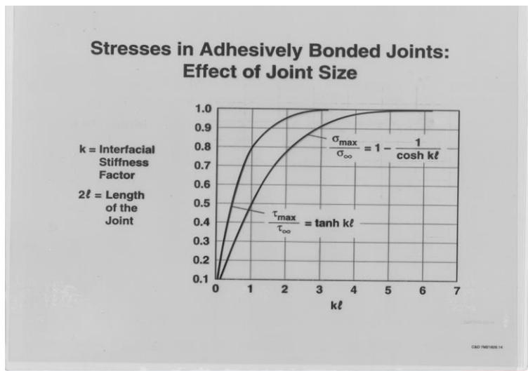
Fig. 4 If the induced stresses are already high, they do not increase with the further increase in the assembly size, if the product  $kl$  of the parameter  $k$  of the interfacial shearing stress and half the assembly length  $l$  exceeds the level  $kl \approx 2.5$ .
