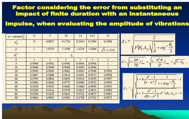
Fig. 18 Error from substituting an impact load of finite duration with an instantaneous impulse
