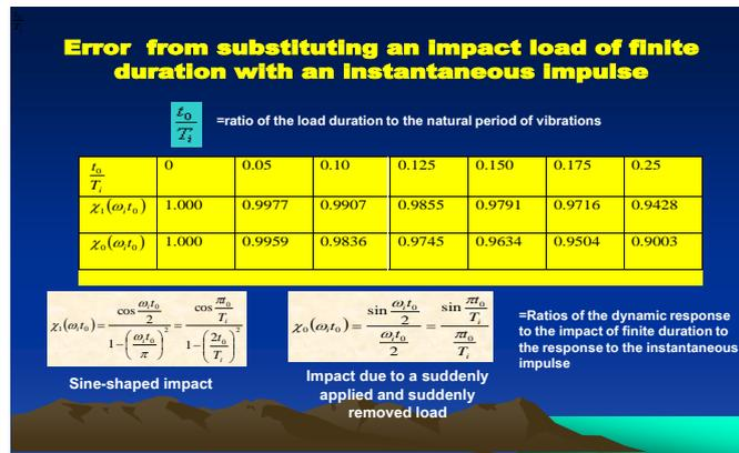
Fig. 17 Factor considering the error from substituting an impact of finite duration with an instantaneous impulse
