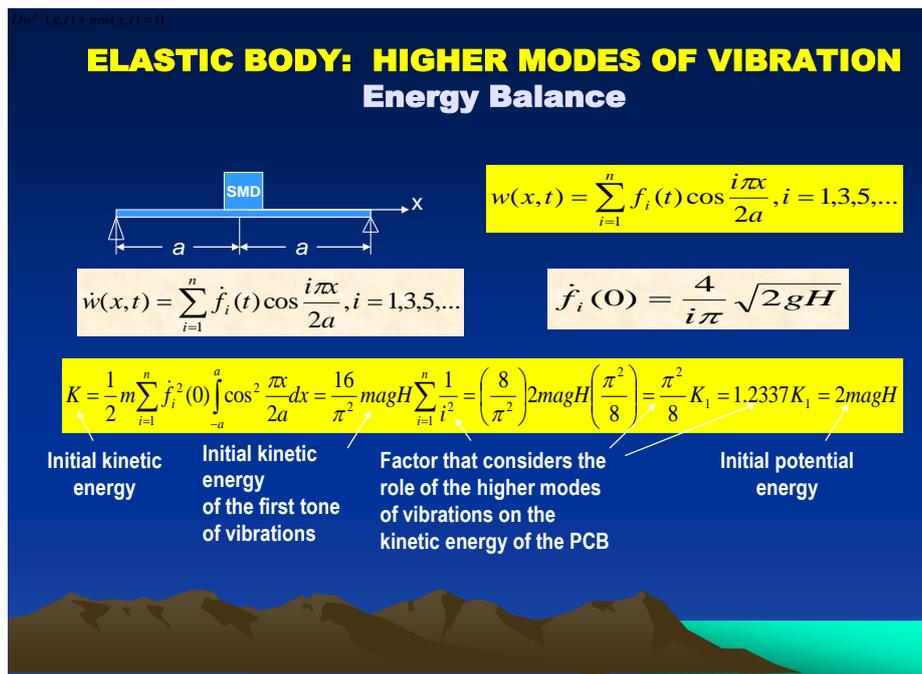
Fig. 11 How significant is the role of higher modes of the induced vibrations?
