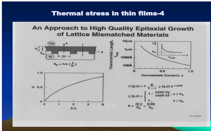
Fig. 7 Novel approach to the high-quality epitaxial growth of lattice-mismatched materials. It was suggested that a semiconductor film was grown on a specially engineered substrate with little “towers” on its surface
