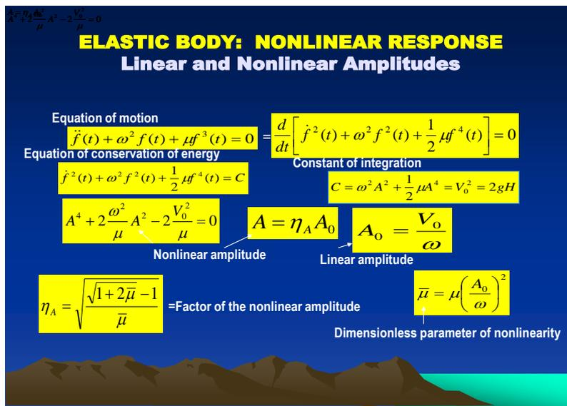
Fig. 14 Nonlinear dynamic response: equation of motion, linear and nonlinear amplitudes
