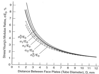
$\sigma_t$  = maximum tensile stress;  $\sigma_e$  = maximum compressive stress;  $\sigma_t^0$  = maximum tensile stress without considering the shift in the centroid;  $\sigma_e^0$  = maximum compressive stress without considering the shift in the centroid,  $E_0$  = nominal (low strain) Young's modulus
