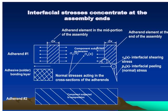
Fig. 2 The segment in the middle of the assembly is equilibrated by the normal stresses only, while the segment at the assembly ends needs interfacial shearing and peeling forces/stresses to be equilibrated
