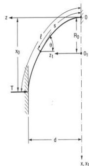
**Optical Fiber “Pigtail” Bent on a Cylindrical Surface**
