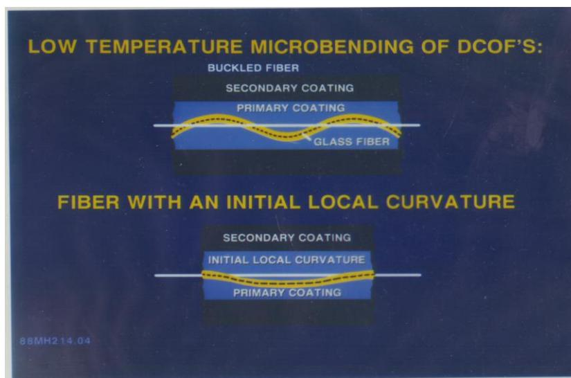
Fig. 20 Low temperature micro-bending of dual-coated optical fibers (Suhir 2014c)
