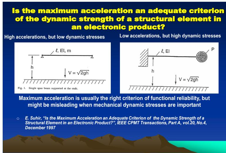
Fig. 8 Structural element idealized as a simply supported beam (on the left) experiences, as a result of drop tests, high accelerations. These are proportional to the frequency of vibrations squared, and the frequency of the drop induced vibrations is high. The induced stresses are, however, low. On the other hand, the cantilever beam with a lump mass at the end experiences high stresses at its clamped end, while the induced frequencies and, hence, the accelerations might be low
