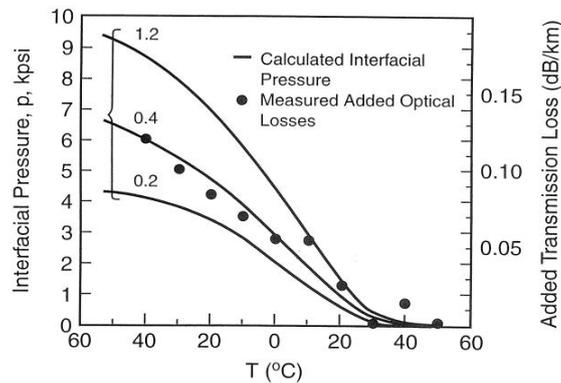
Fig. 19 Calculated pressures and measured added optical losses vs. temperature in jacketed optical fibers
