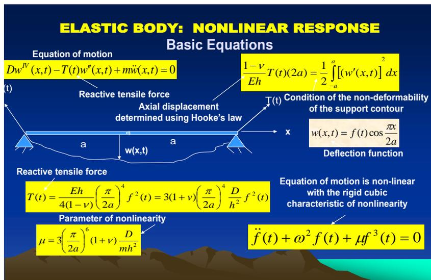
Fig. 13 Nonlinear dynamic response of a PCB to a shock load
