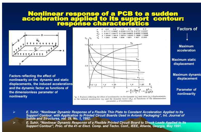
Fig. 15 Nonlinear response of a PCB to a sudden constant acceleration applied to its support contour
