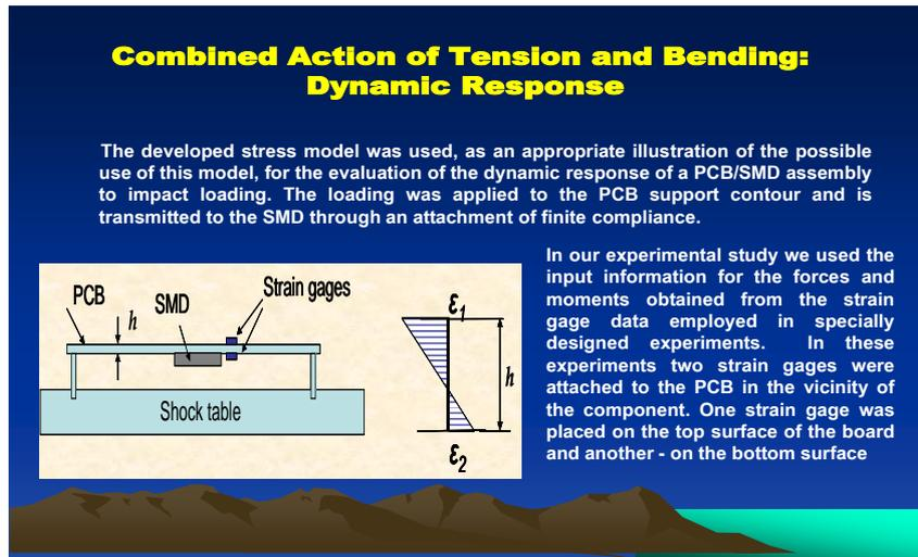
Fig. 9 Experimental setup for drop tests
