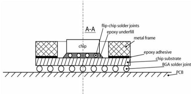
Fig. 1 Typical microelectronic package design. The surrogate metal frame is introduced to keep the package flat during processing and operation. The induced stresses in the package materials could be, however, quite high
