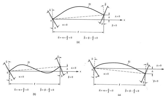
Fig. 22 Optical fiber interconnect subjected to the ends offset
