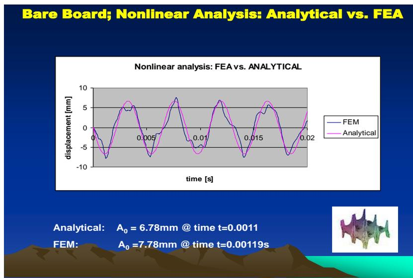
Fig. 12 Analytical vs. FEA data for the nonlinear dynamic response of a PCB to a drop impact
