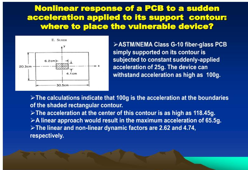
Fig. 16 The vulnerable electronic device should be placed outside the shaded area
