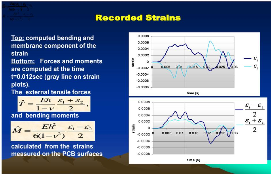
Fig. 10 Combined action of tensile and bending deformations (left sketch) and the recorded normal strains on both sides of the PCB (right sketch)
