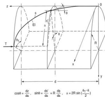
Fig. 21 Optical fiber pigtail configured as a quarter of a circumference (a) and optimized configurations of an optical fiber pigtail for undersea applications (b)
