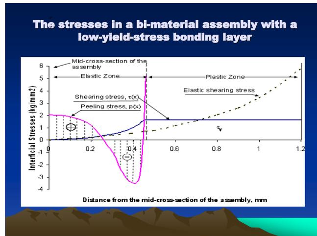
Fig. 5 The interfacial shearing stress increases at the assembly mid-portion from zero at the assembly mid-cross-section to its yield value, and then remains equal to the yield stress in shear
