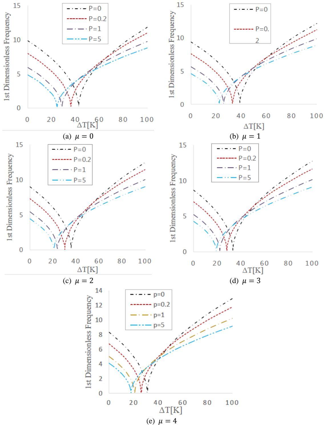
Fig. 5 Variations of the first dimensionless natural frequency of the FG nanobeam with respect to uniform temperature change for different values of power-law exponent and nonlocal parameters ( $L/h = 20$ )
