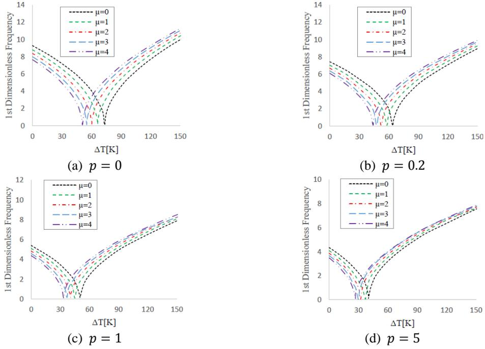
Fig. 16 Variations of the first dimensionless natural frequency of the FG nanobeam with respect to non-linear temperature change for different values of nonlocal parameters and power-law exponents ( $L/h = 50$ )
