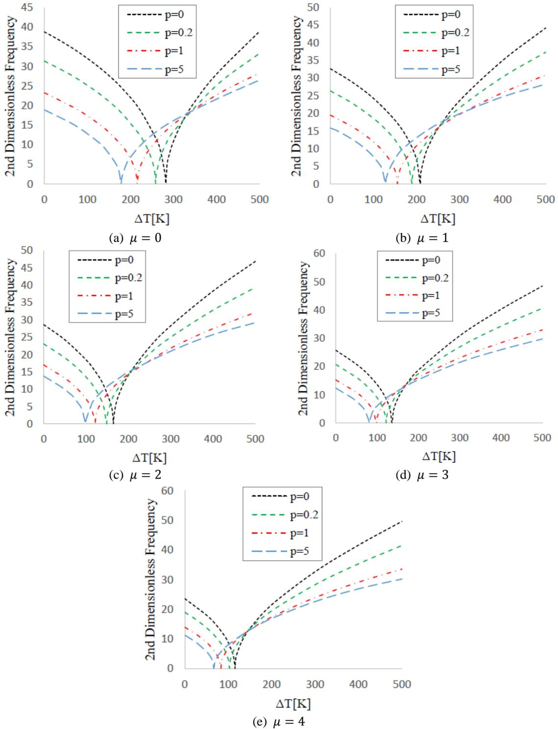
Fig. 10 Variations of the second dimensionless natural frequency of the FG nanobeam with respect to non-linear temperature change for different values of power-law exponents and nonlocal parameters ( $L/h = 50$ )
