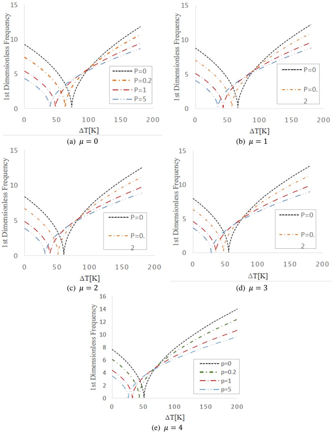
Fig. 6 Variations of the first dimensionless natural frequency of the FG nanobeam with respect to linear temperature change for different values of power-law exponent and nonlocal parameters ( $L/h = 25$ )
