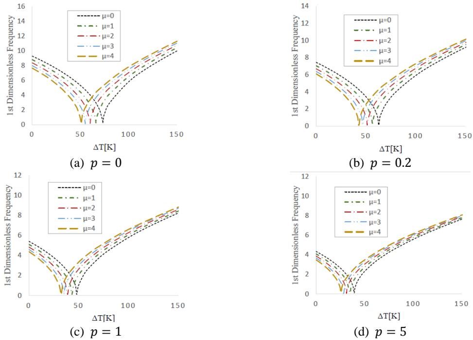
Fig. 15 Variations of the first dimensionless natural frequency of the FG nanobeam with respect to linear temperature change for different values of nonlocal parameters and power-law exponents ( $L/h = 50$ )
