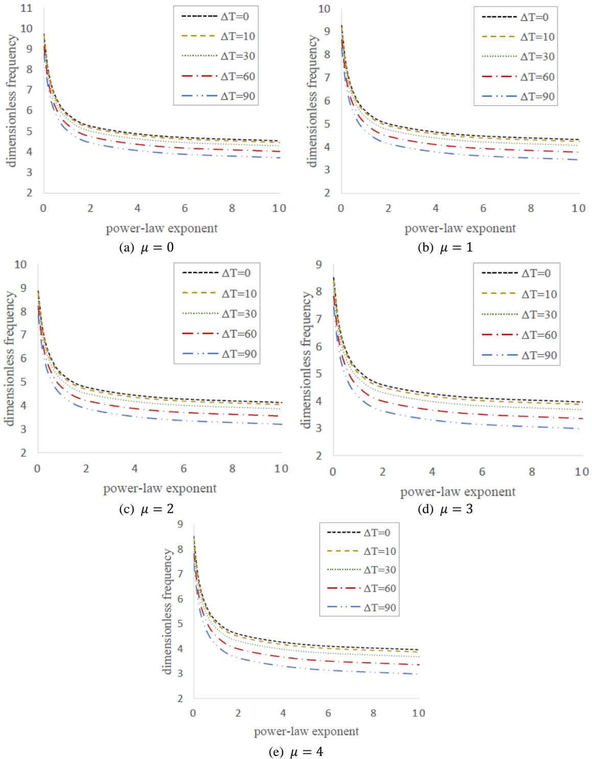
Fig. 3 The variation of the first dimensionless frequency of the FG nanobeam under linear temperature change with power-law exponent and temperature rises for different nonlocal parameters ( $L/h = 20$ )
