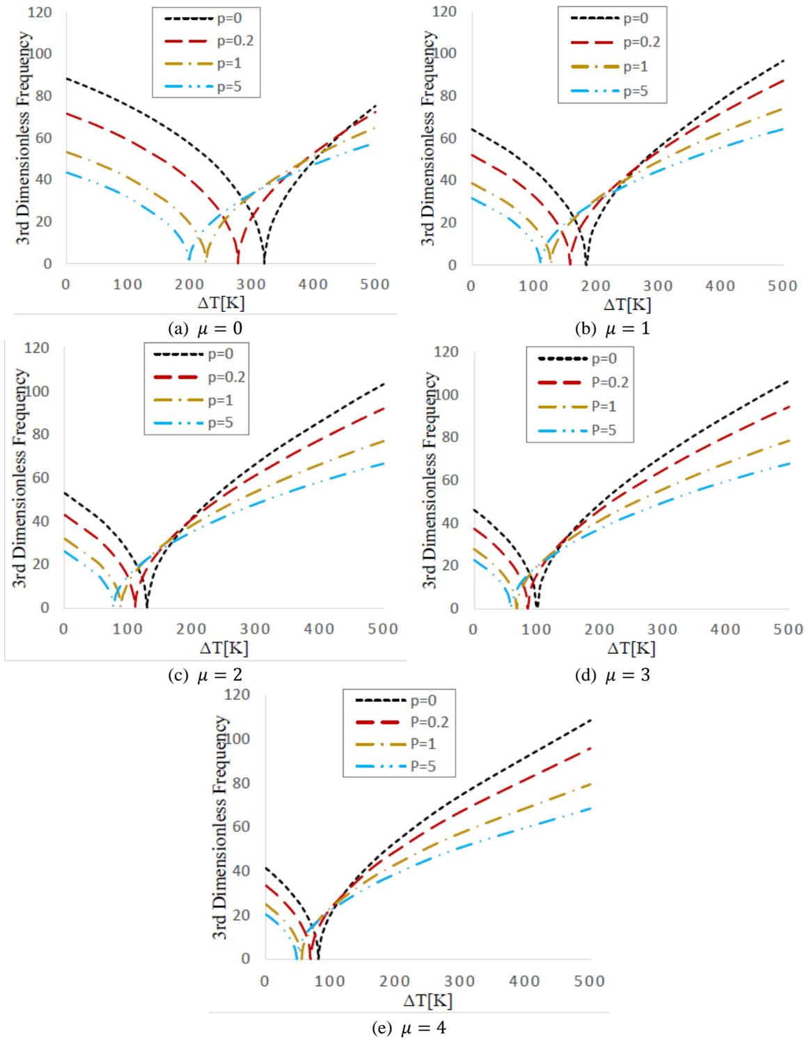
Fig. 11 Variations of the third dimensionless natural frequency of the FG nanobeam with respect to uniform temperature change for different values of gradient indexes and nonlocal parameters ( $L/h = 50$ )
