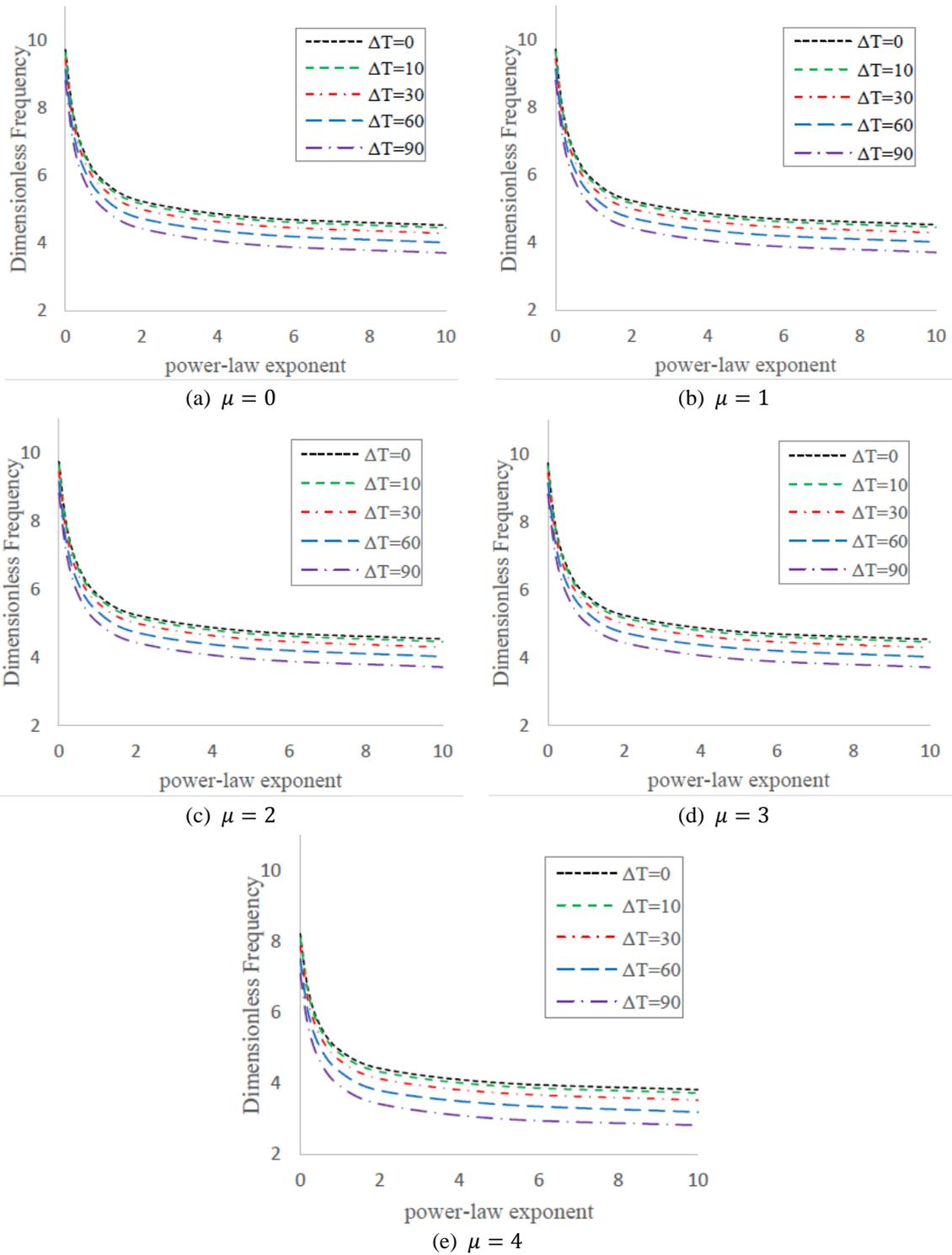
Fig. 4 The variation of the first dimensionless frequency of FG nanobeam under non-linear temperature change for different nonlocal parameters ( $L/h = 20$ )
