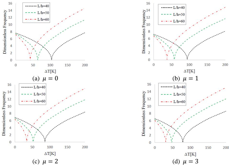
Fig. 19 Variations of the first dimensionless natural frequency of the FG nanobeam with respect to non-linear temperature change for different values of slenderness ratios and nonlocal parameters
