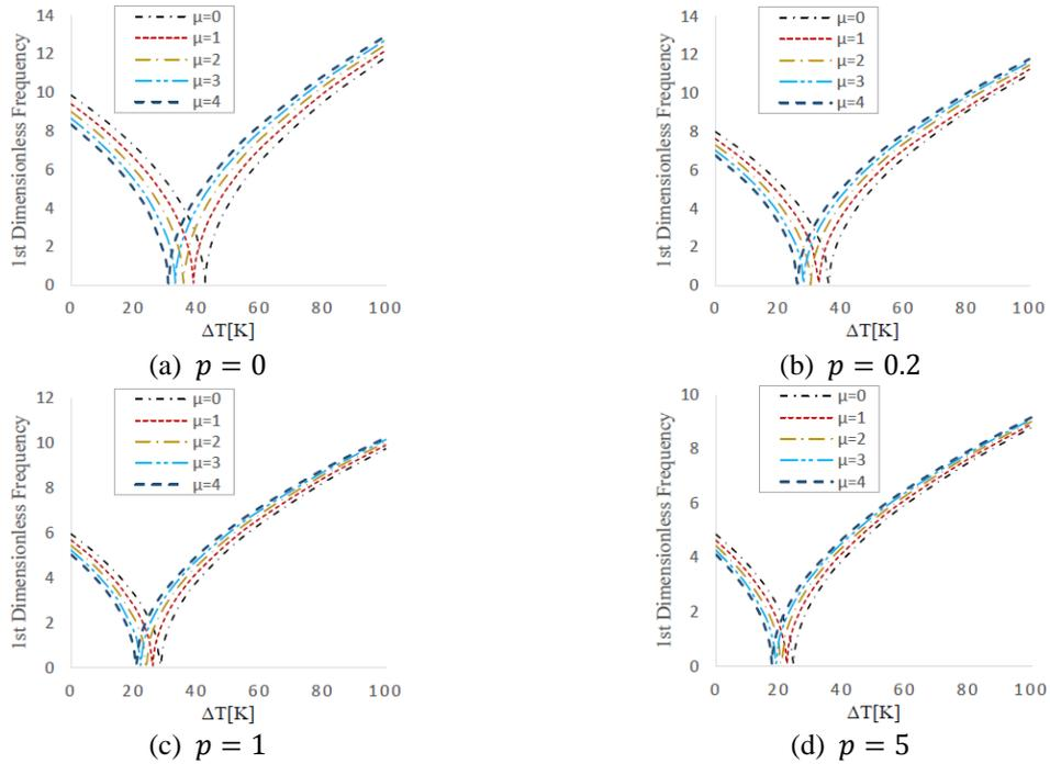
Fig. 14 Variations of the first dimensionless natural frequency of the FG nanobeam with respect to uniform temperature change for different values of nonlocal parameters and power-law exponents ( $L/h = 50$ )
