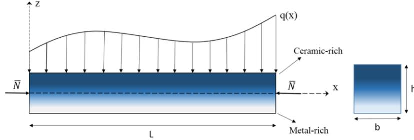
Fig. 1 Geometry and coordinates of FG nanobeam
