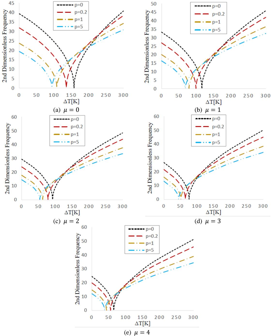
Fig. 7 Variations of the first dimensionless natural frequency of the FG nanobeam with respect to non-linear temperature change for different values of power-law exponent and nonlocal parameters ( $L/h = 50$ )
