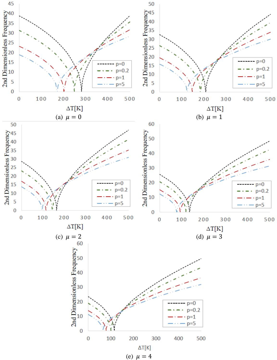
Fig. 9 Variations of the second dimensionless natural frequency of the FG nanobeam with respect to linear temperature change for different values of power-law exponents and nonlocal parameters ( $L/h = 50$ )
