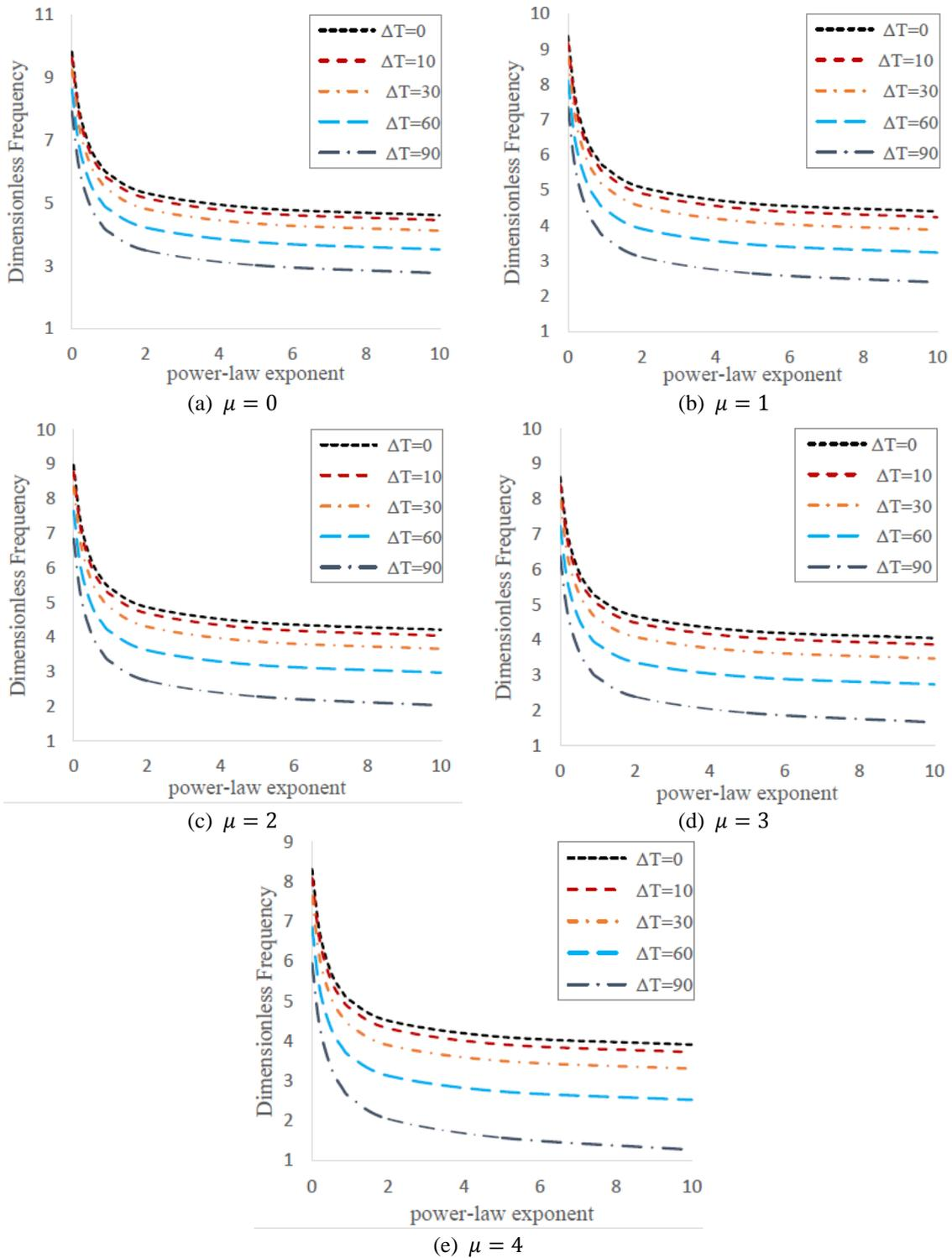
Fig. 2 The variation of the first dimensionless frequency of the FG nanobeam under uniform temperature change with power-law exponent and temperature rises for different nonlocal parameters ( $L/h = 20$ )
