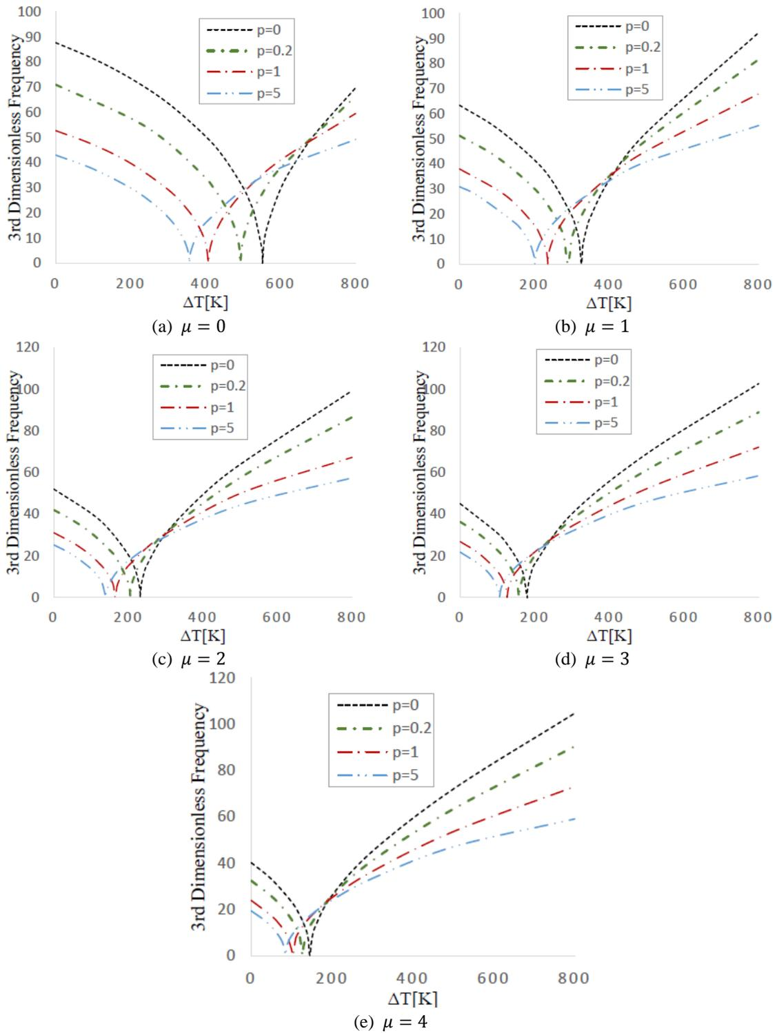
Fig. 12 Variations of the third dimensionless natural frequency of the FG nanobeam with respect to linear temperature change for different values of gradient indexes and nonlocal parameters ( $L/h = 50$ )
