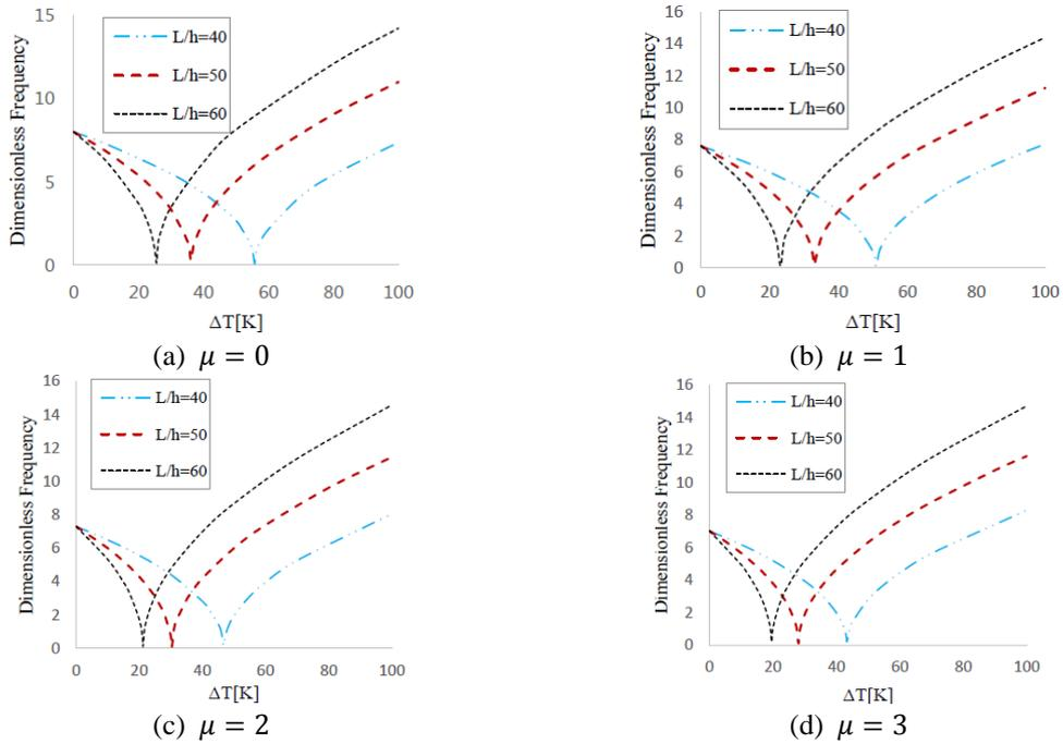
Fig. 17 Variations of the first dimensionless natural frequency of the FG nanobeam with respect to uniform temperature change for different values of slenderness ratios and nonlocal parameters ( $p = 0.2$  and  $L/h = 50$ )
