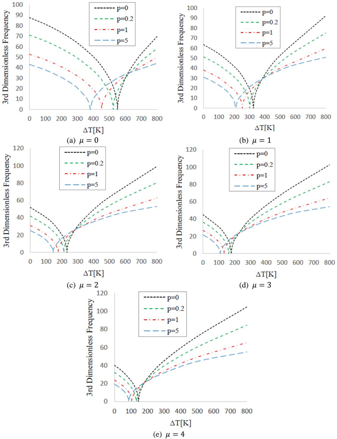
Fig. 13 Variations of the third dimensionless natural frequency of the FG nanobeam with respect to non-linear temperature change for different values of gradient indexes and nonlocal parameters ( $L/h = 50$ )
