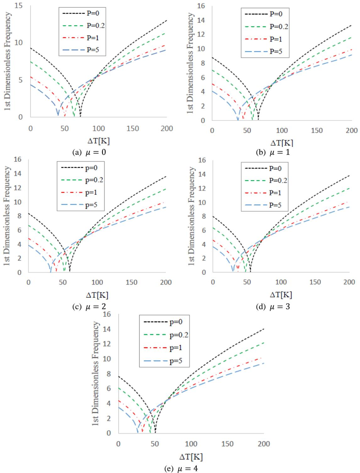
Fig. 8 Variations of the second dimensionless natural frequency of the FG nanobeam with respect to uniform temperature change for different values of power-law exponents and nonlocal parameters ( $L/h = 50$ )
