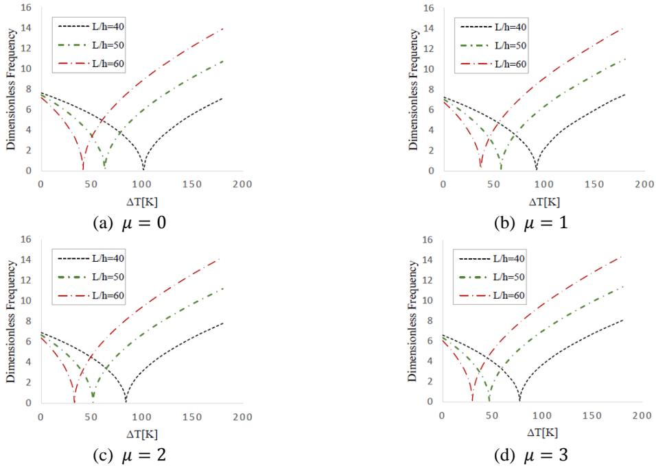
Fig. 18 Variations of the first dimensionless natural frequency of the FG nanobeam with respect to linear temperature change for different values of slenderness ratios and nonlocal parameters ( $p = 0.2$  and  $L/h = 50$ )
