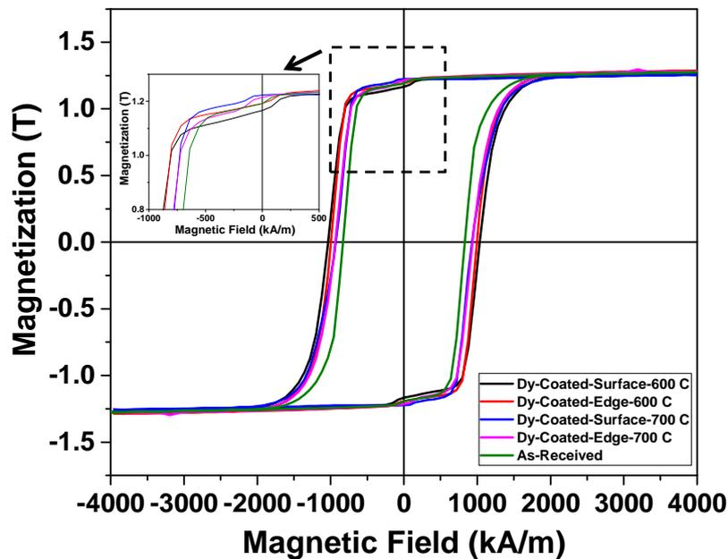
Fig. 2 Hysteresis loops after sputter deposition of Dy films onto both edges and whole surface of the magnet followed by post-annealing at 600 and 700 °C
