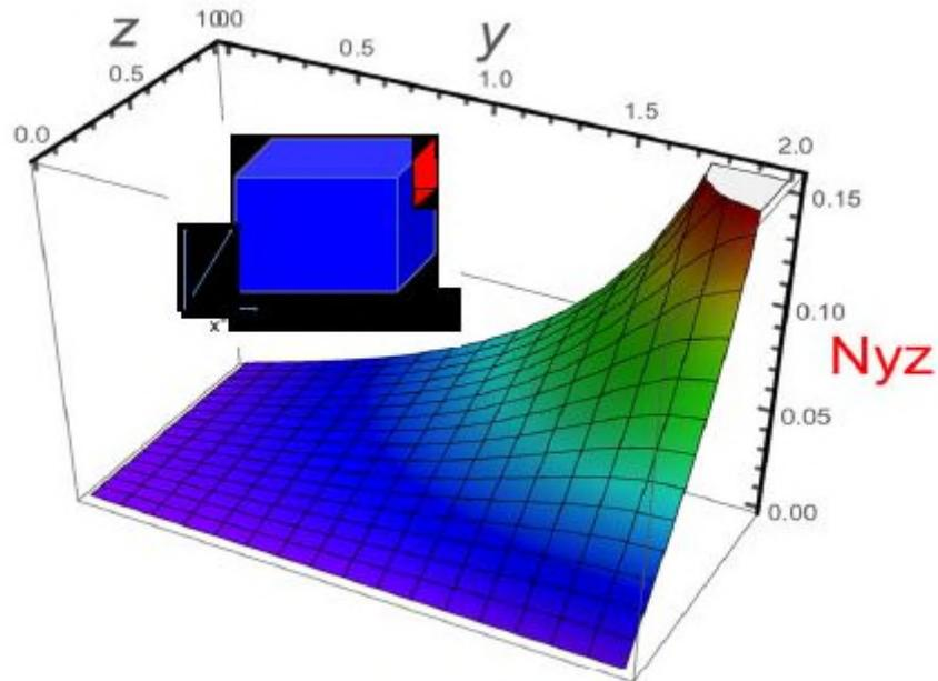
Fig. 4 The calculated demagnetization factor  $N_{yz}$  along the  $x=a$  (side) surface of the body indicated in the inset.
