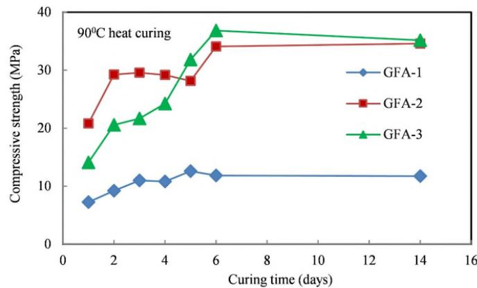
Fig. 4 Compressive strength variation with age for fly ash geopolymer mortar heat cured at 90°C
