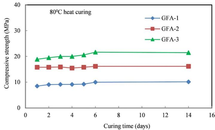
Fig. 5 Compressive strength variation with age for fly ash geopolymer mortar heat cured at 80°C
