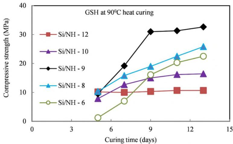
Fig. 7 Compressive strength variation with Si/OH for Shirasu geopolymer mortar
