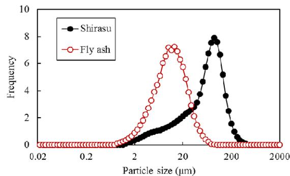
Fig. 1 Particle size distribution of aluminosilicates
