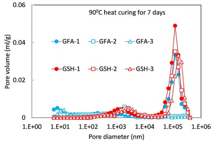
Fig. 6 Pore distribution of all geopolymer mortars subjected to temperature of 90°C up to 7 days
