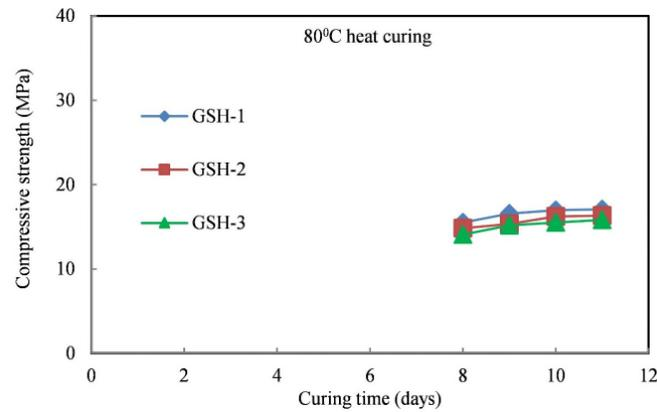
Fig. 3 Compressive strength variation with age for Shirasu geopolymer mortar heat cured at 80°C
