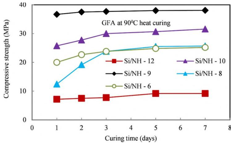
Fig. 8 Compressive strength variation with Si/OH for fly ash geopolymer mortar
