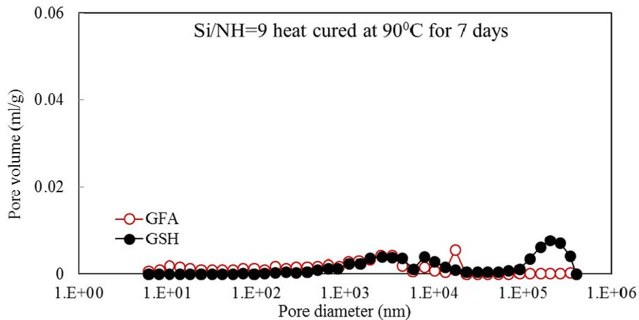
Fig. 9 Pore distribution of all geopolymer mortars subjected to temperature of 90°C up to 7 days for mix with Si/NH=9
