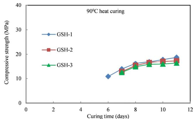
Fig. 2 Compressive strength variation with age for Shirasu geopolymer mortar heat cured at 90°C
