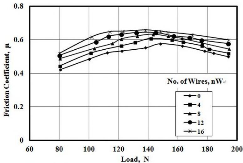
Fig. 13 Effect of number of wires on friction coefficient,  $diW = 0.7$  mm and  $dsW = 4$  mm
