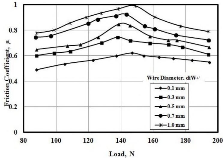
Fig. 12 Effect of wire diameter on friction coefficient,  $dsW = 4$  mm and  $nW = 16$  wires
