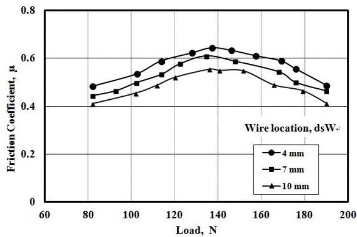
Fig. 16 Effect of wire location on friction coefficient,  $diW = 0.5$  mm and  $nW = 8$  wires
