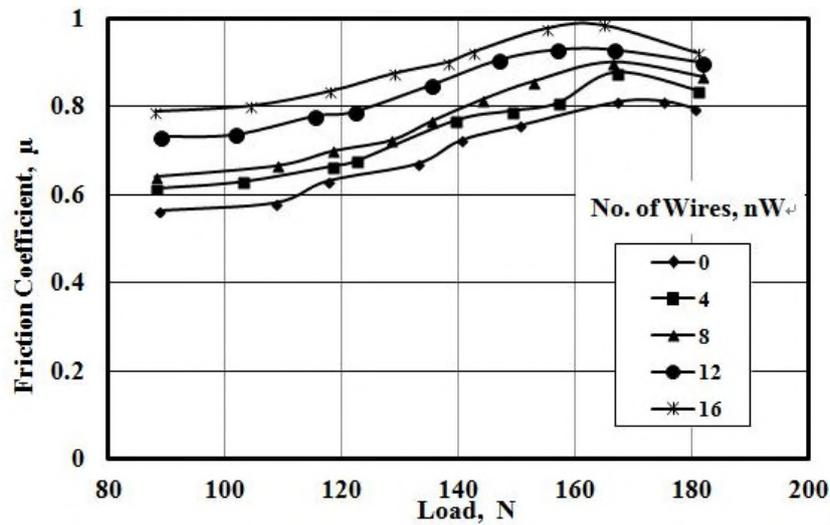
Fig. 3 Effect of number of wires on friction coefficient,  $d_iW=0.3\text{mm}$  and  $d_sW=7\text{mm}$
