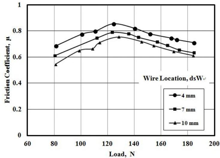
Fig. 10 Effect of wire location on friction coefficient,  $diW = 0.3$  mm and  $nW = 16$  wires
