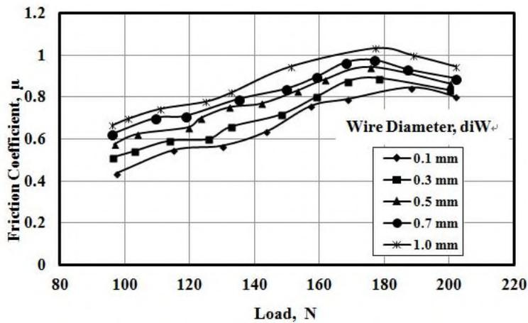
Fig. 7 Effect of wire diameter on friction coefficient,  $dsW = 4\text{mm}$  and  $nW = 16$  wires
