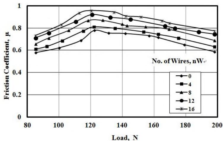
Fig. 9 Effect of number of wires on friction coefficient,  $d_iW = 0.7\text{mm}$  and  $d_sW = 4\text{mm}$
