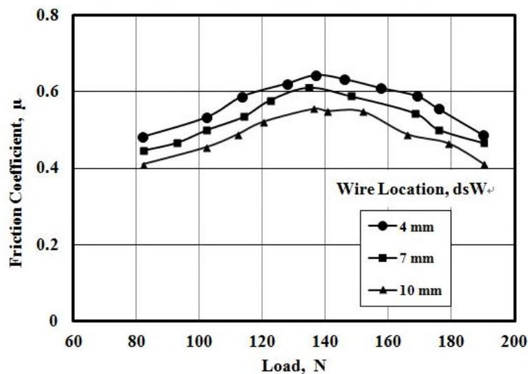
Fig. 14 Effect of number of wires on friction coefficient,  $d_iW = 0.3$  mm and  $d_sW = 4$  mm
