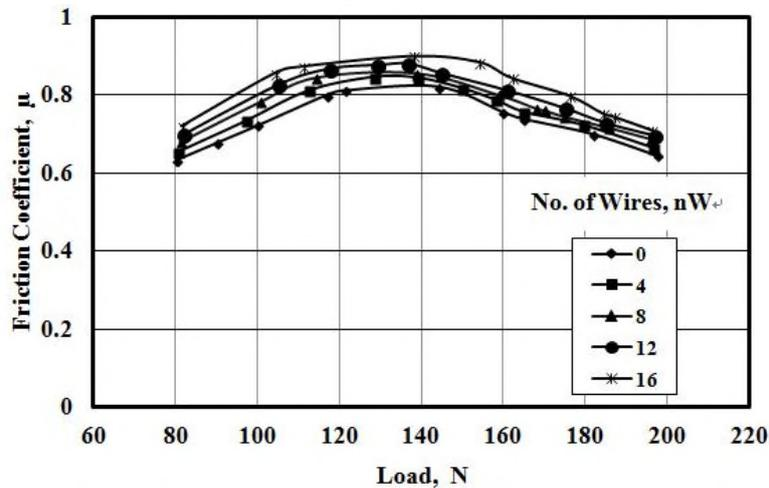
Fig. 8 Effect of number of wires on friction coefficient,  $d_iW = 0.5\text{mm}$  and  $d_sW = 7\text{mm}$
