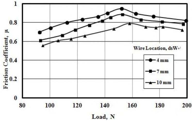
Fig. 5 Effect of wire location on friction coefficient,  $diW = 0.3\text{mm}$  and  $nW = 8$  wires
