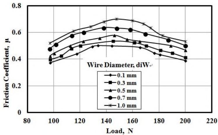
Fig. 17 Effect of wire diameter on friction coefficient,  $nW = 16$  wires and  $dsW = 4$  mm
