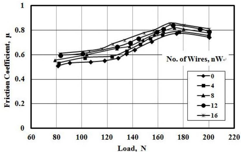
Fig. 4 Effect of number of wires on friction coefficient,  $d_iW=0.5\text{ mm}$  and  $d_sW=7\text{ mm}$
