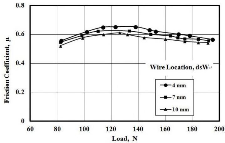
Fig. 15 Effect of wire location on friction coefficient,  $diW = 0.7$  mm and  $nW = 16$  wires
