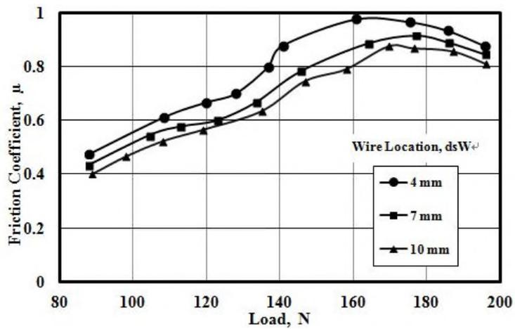
Fig. 6 Effect of wire location on friction coefficient,  $diW = 1.0\text{mm}$  and  $nW = 8$  wires
