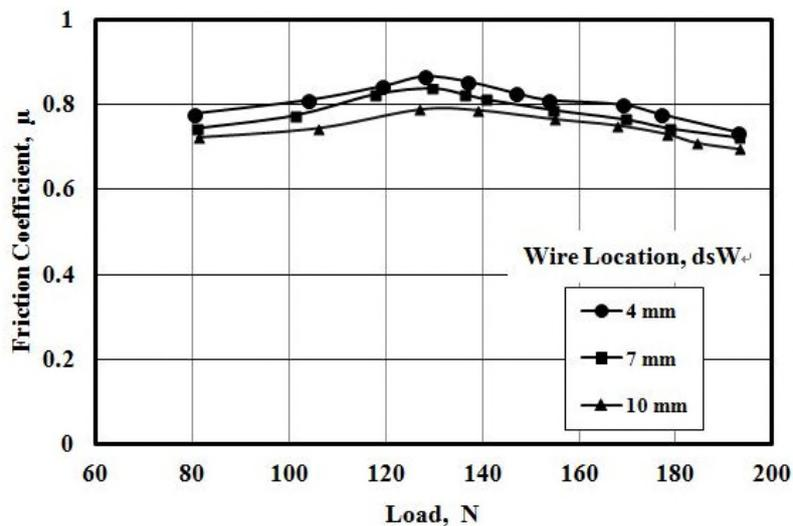
Fig. 11 Effect of wire location on friction coefficient,  $diW = 0.5$  mm and  $nW = 12$  wires
