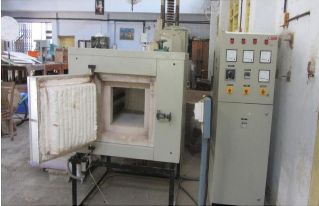
Fig. 1 Programmable electric furnace
