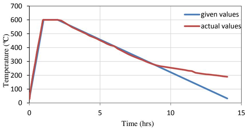
Fig. 5 Furnace performance at 600°C and no charge
