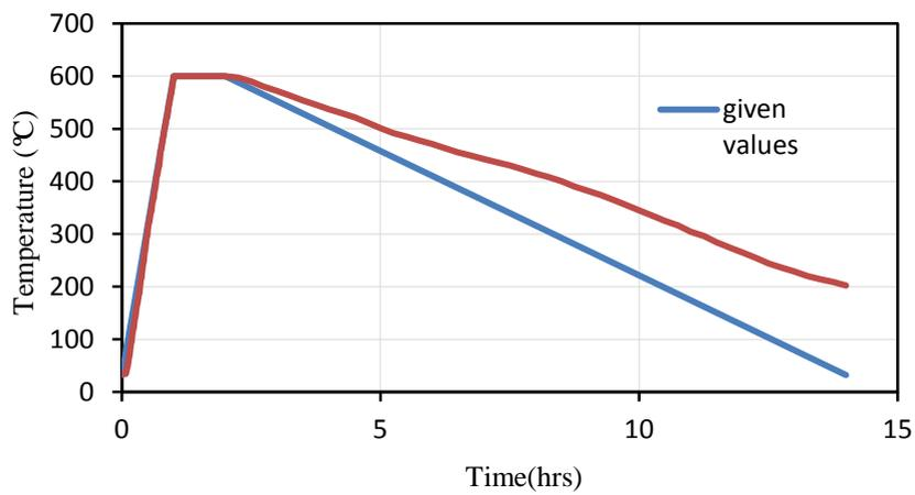
Fig. 8 Furnace performance at 600°C with 40kg charge
