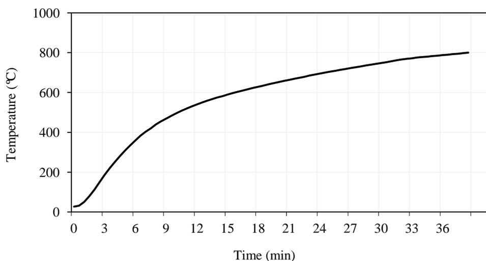
Fig. 2 Maximum rate of heating of furnace with no charge
