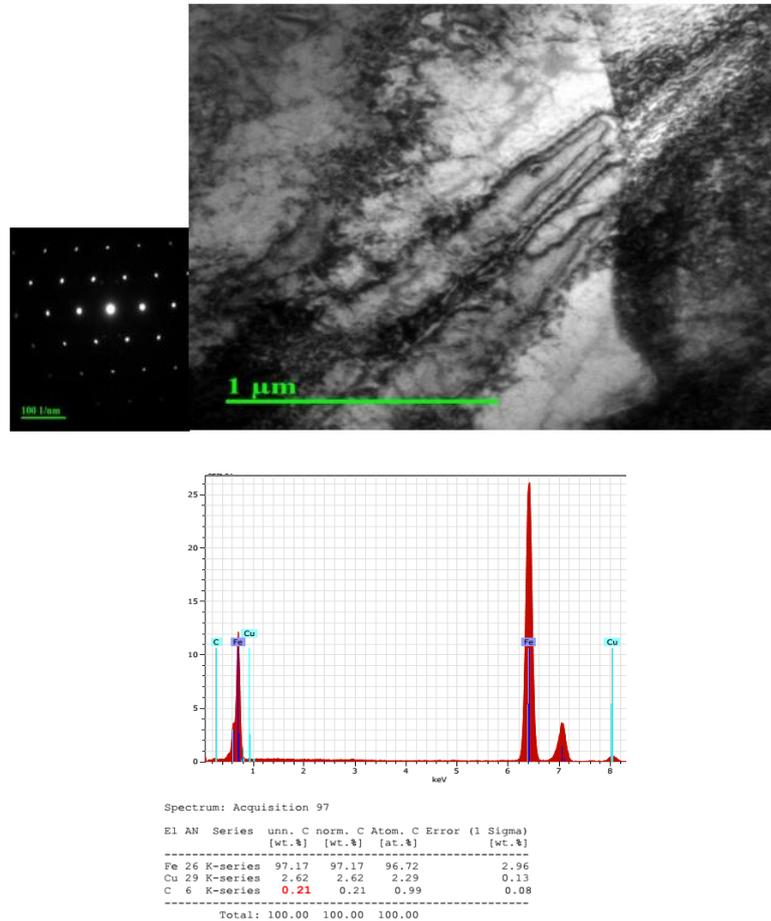
Fig. 9 Transmission electron micrograph shows ferrite crystal with embedded martensite; SADP of the area typifies bcc ferrite and ferrite adjoining martensite is seen to contain dislocations. EDX shows 0.2 wt% C in martensite
