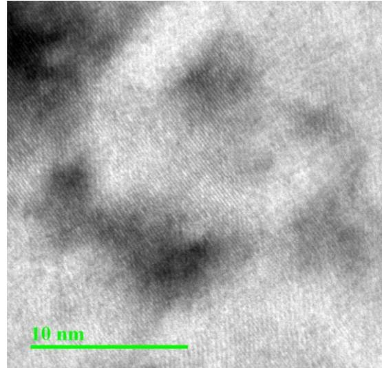
Fig. 13 Lattice image of steel as in Fig. 12 shows evidence of carbide nuclei
