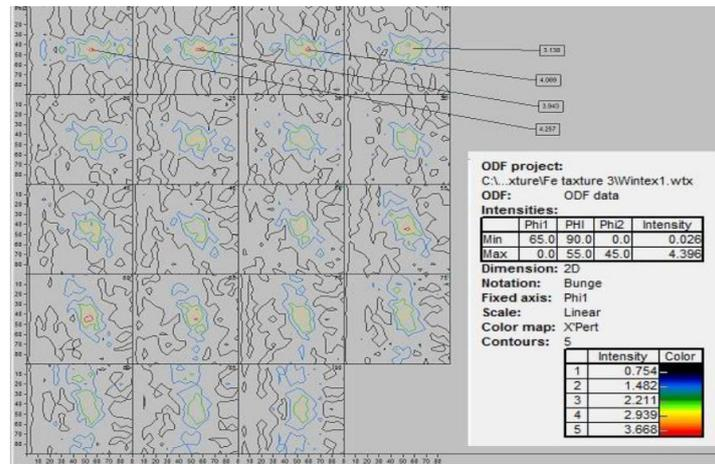
Fig. 16 ODF of steel annealed at 800°C
