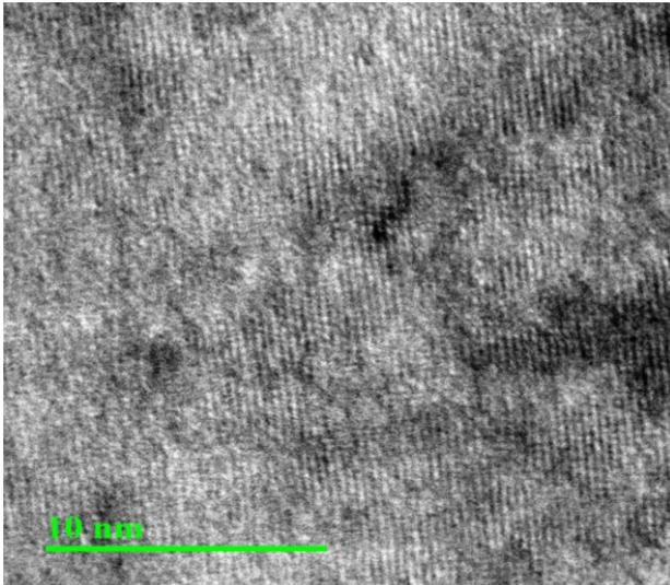
Fig. 12 Lattice image of steel annealed at 750°C
