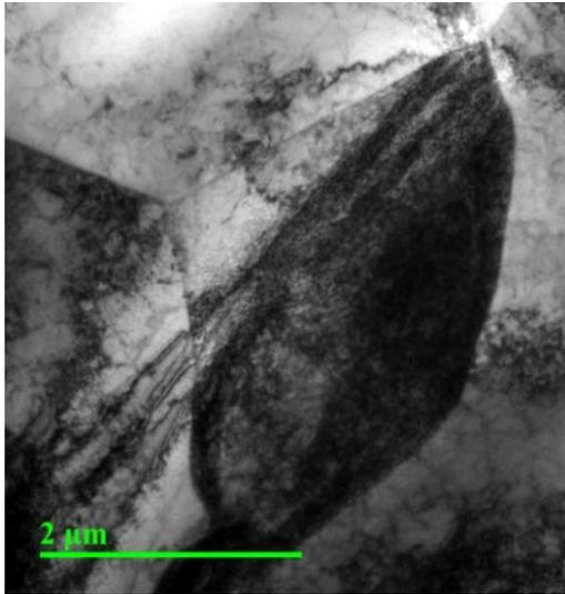
Fig. 10 Martensite in ferrite matrix, BF
