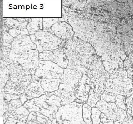
Fig. 4 Optical microstructure of steel annealed at 800°C
