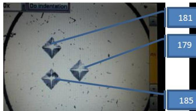
Fig. 7(b) Microhardness results of steel annealed at 675°C for 2h
