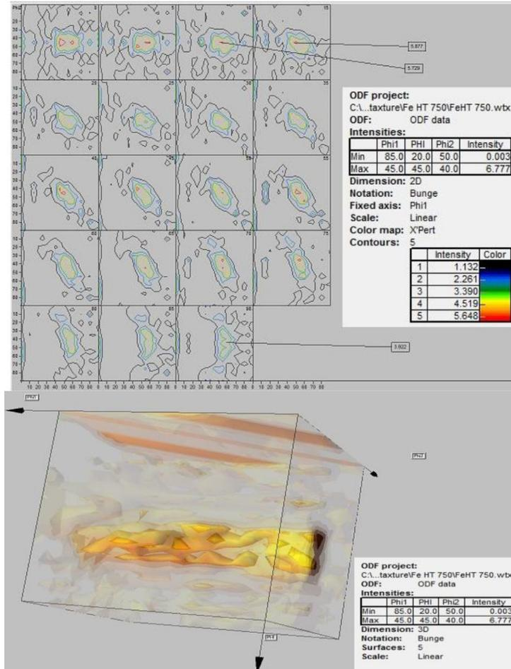
Fig. 15 ODF of steel annealed at 750°C
