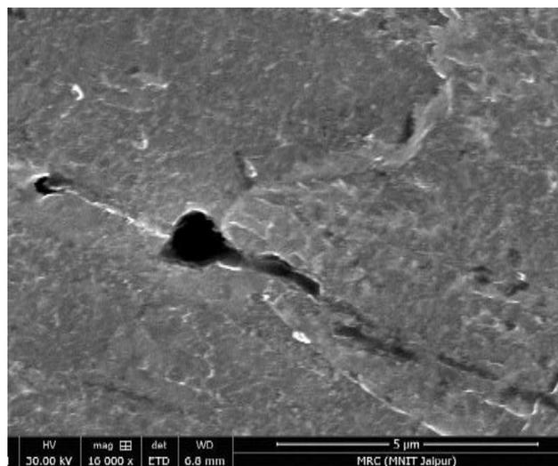
Fig. 8 Scanning electron micrograph of steel annealed at 700°C
