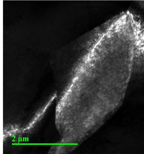
Fig. 11 Dark field photograph of martensite
