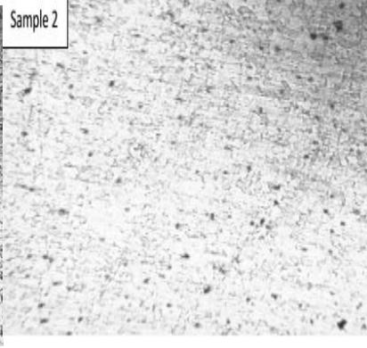
Fig. 3 Optical microstructure of steel annealed at 775°C
