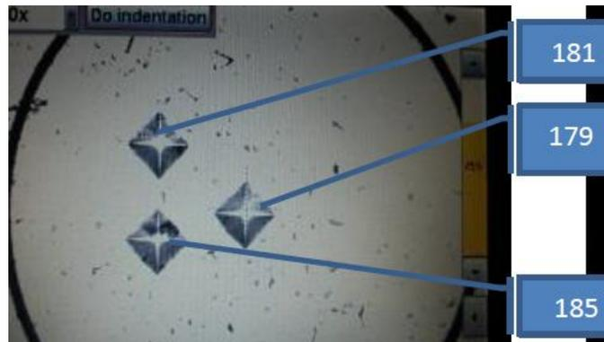
Fig. 7(a) Microhardness results of steel annealed at 750°C
