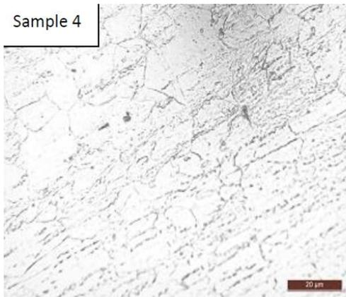
Fig. 5 Optical microstructures of steel annealed at 675°C for 1hr
