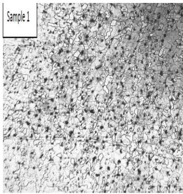
Fig. 2 Optical microstructure of steel annealed at 750°C
