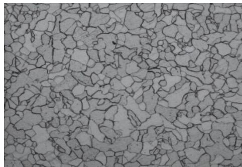
Fig. 1 Microstructure of experimental steel annealed in received condition (Normalized)
