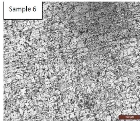
Fig. 6 Optical microstructures of steel annealed at 675°C for 4 hrs
