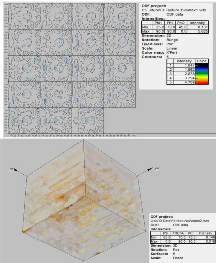
Fig. 14 ODF of as received IF steel; three dimensional ODF is shown
