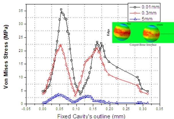
Fig. 9. Variation of the stress in cement around the mobile cavity according to the distance separating it to that fixed at the free edge both to the interface cement/bone
