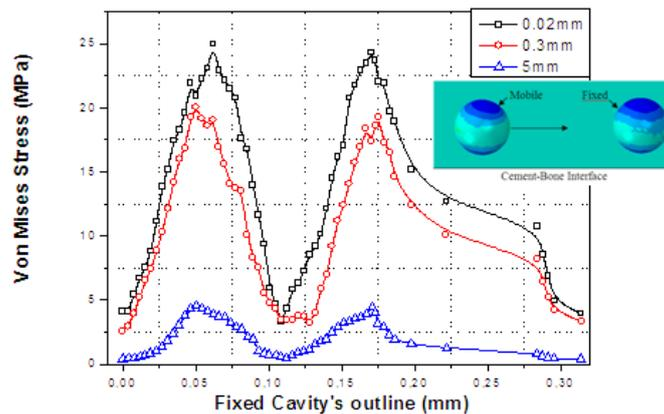
Fig. 11 Variation of the stress around the mobile's cavity according to the distance separating it to that fixed both at the interface cement/bone
