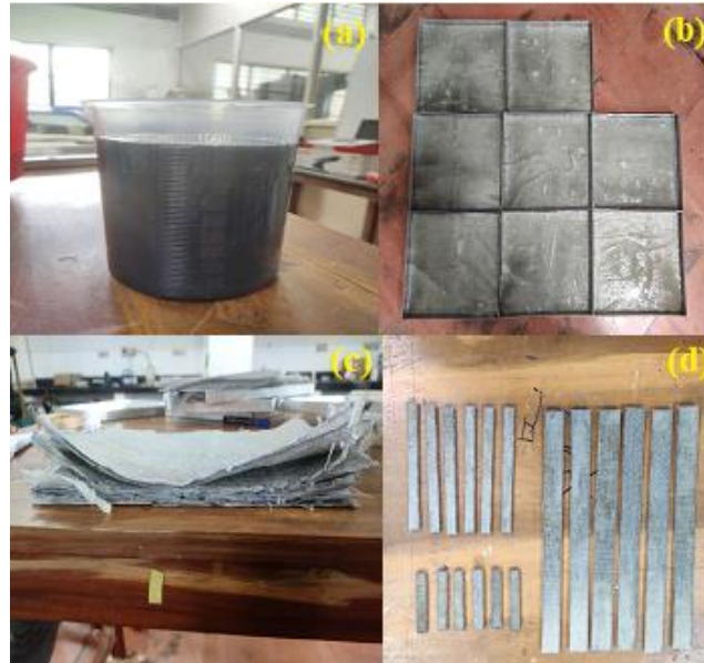
Fig. 7 PLA-Flax fiber with EPO and Graphene Composite Preparation; (a) PLA-EPO-Graphene solution; (b) PrePrep Preparation; (c) Prepreg sheets after drying; (d) Specimens for Testing
