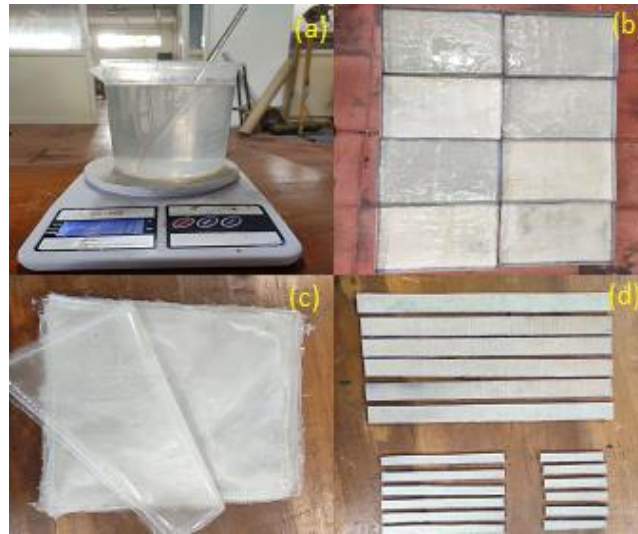
Fig. 5 PLA/Flax Composite Preparation; (a) PLA-Chloroform solution; (b) PrePreg Preparation; (c) Prepreg sheets after drying; (d) Specimens for Testing
