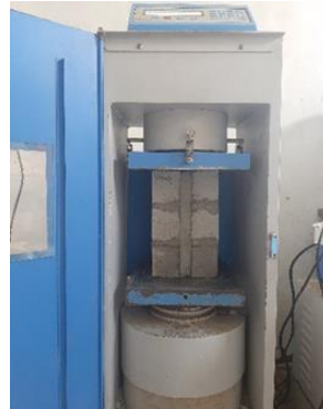
Fig. 6 Test set-up for compression of specimens
