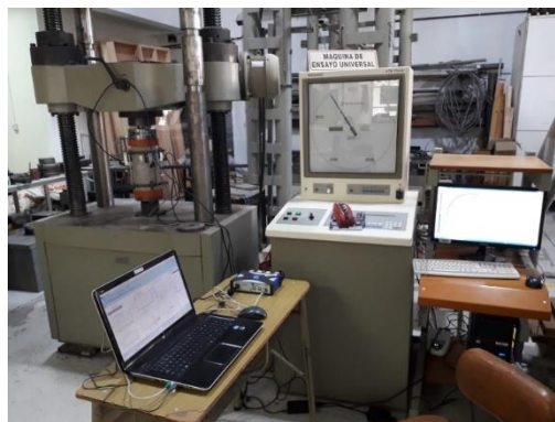
Fig. 1 Simple compression test (Test setup)
